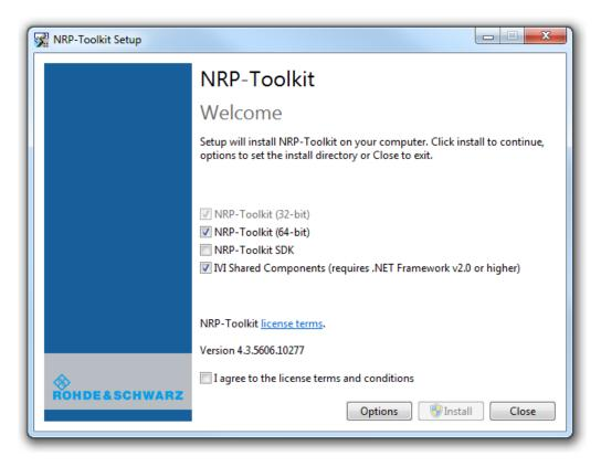
The basic package(s) with the low-level drivers (Kernel modules) need to be installed always. If you plan to develop individual programs, the SDK option (Software Development Kit) should also be selected. This provides header-files, link libraries and example source code for programmers -- these parts will be installed in C:\ProgramData\Rohde-Schwarz\NRP-Toolkit-SDK.
