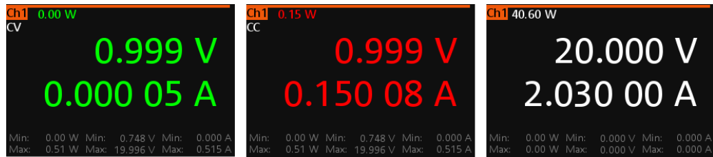
Figure 3-10: Color coding of difference operating conditions
