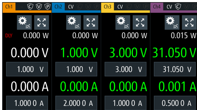
Figure 5-7: Delay text at channel display area
