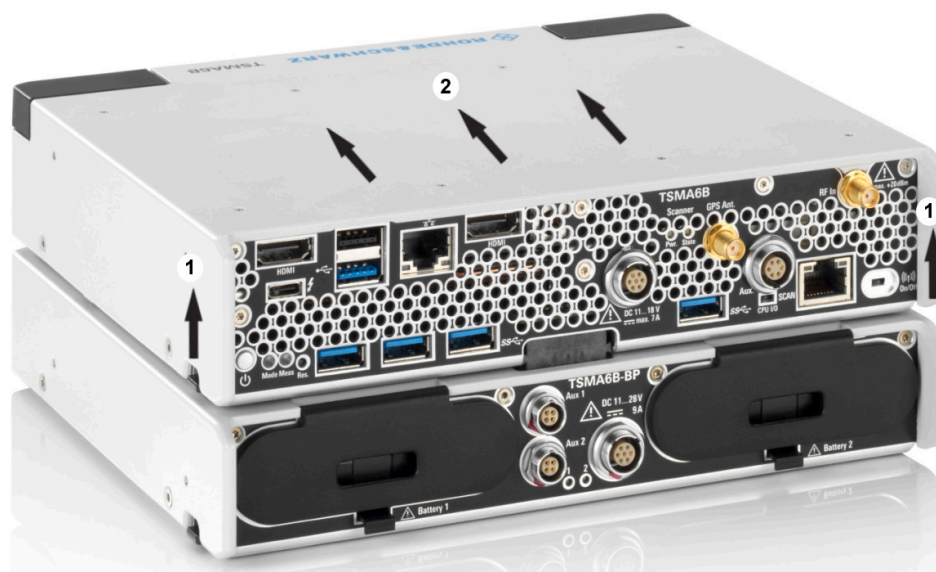
Figure 7-5: Disconnect R&S TSMAX6/6B
