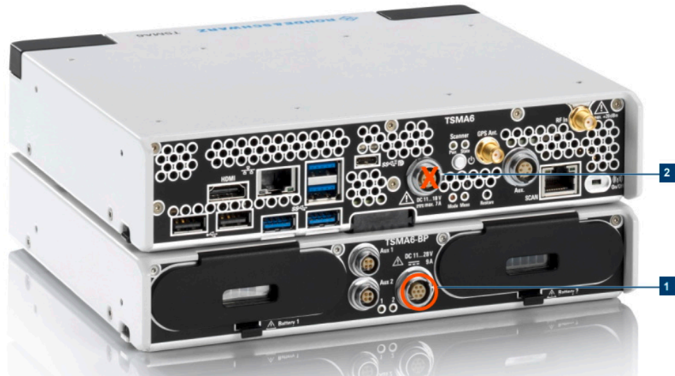
Figure 3-2: DC IN connectors
