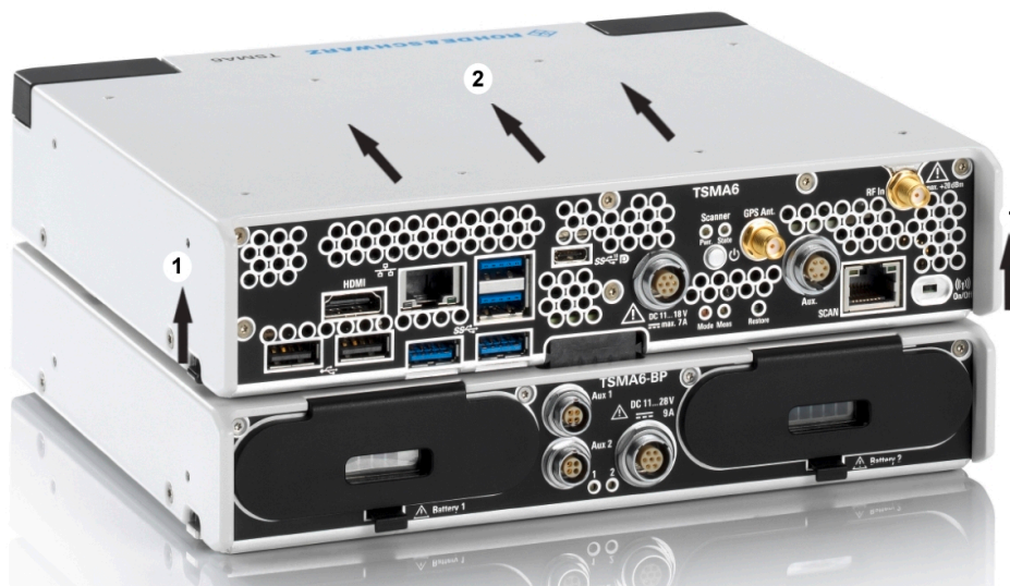
Figure 7-5: Disconnect R&S TSMa6/6B
