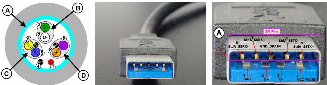
Figure 14-30: USB 3.1 cable cross-section and Standard-A plug - backward compatible with USB 2.0
