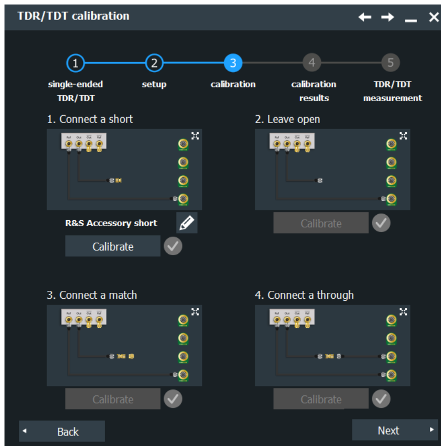
Figure 17-5: Calibration of differential TDR/TDT
