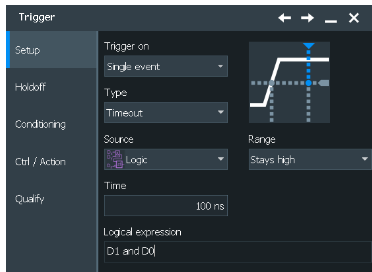
Figure 15-3: Timeout trigger settings for trigger source = logical combination of digital channels
