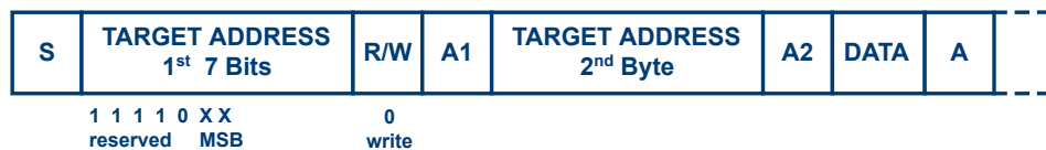
Figure 14-2: 10-bit address, write access
