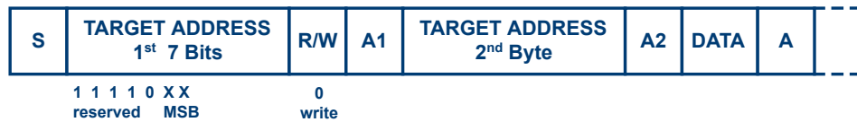
Figure 13-7: 10-bit address, write access
