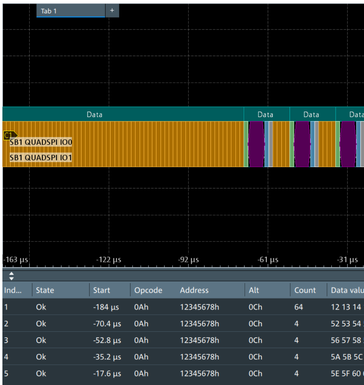
Figure 13-5: Decoded QUAD-SPI signal
