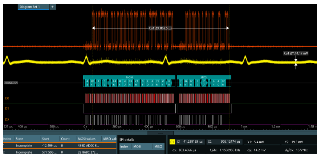
Figure 13-3: Decoded and binary SPI signal
