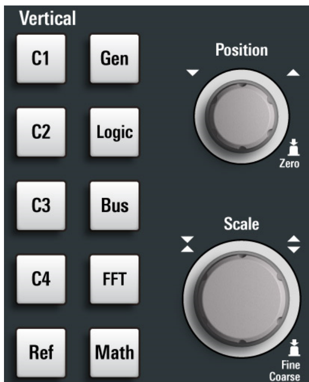
Figure 4-7: Vertical controls of MXO 5C with 4 input channels
