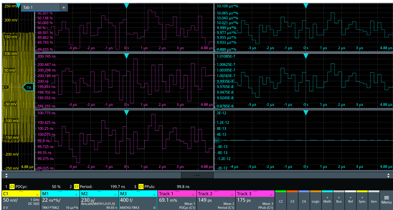
Figure 9-7: Tracks used in math functions
