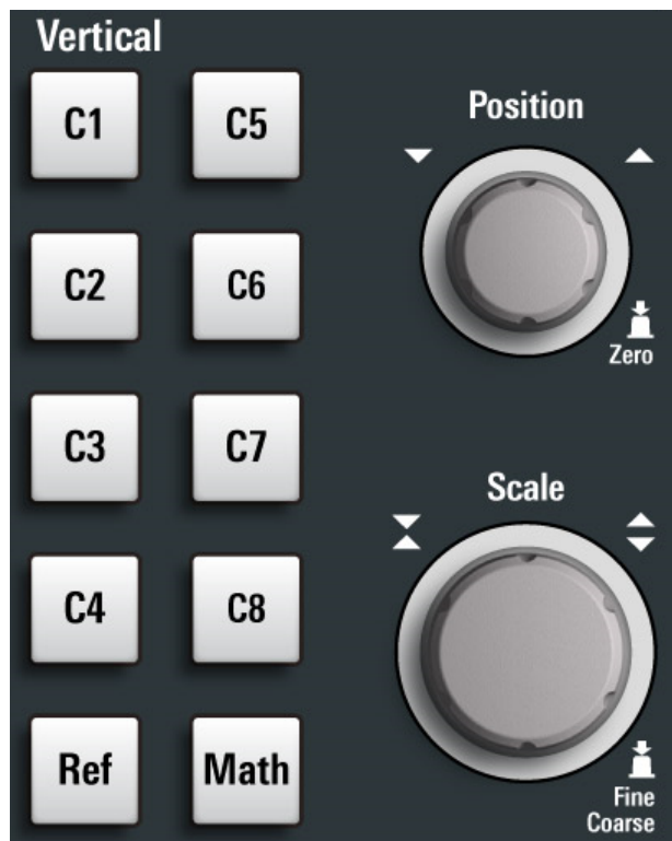
Figure 3-5: Vertical controls of MXO 5 with 8 input channels
