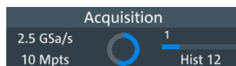
Figure 4-9: Progress of incomplete long acquisition in average mode, Run Single = 5, first acquisition is finished
