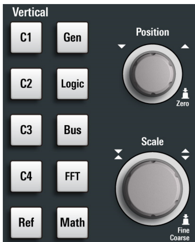
Figure 3-4: Vertical controls of MXO 5 with 4 input channels
