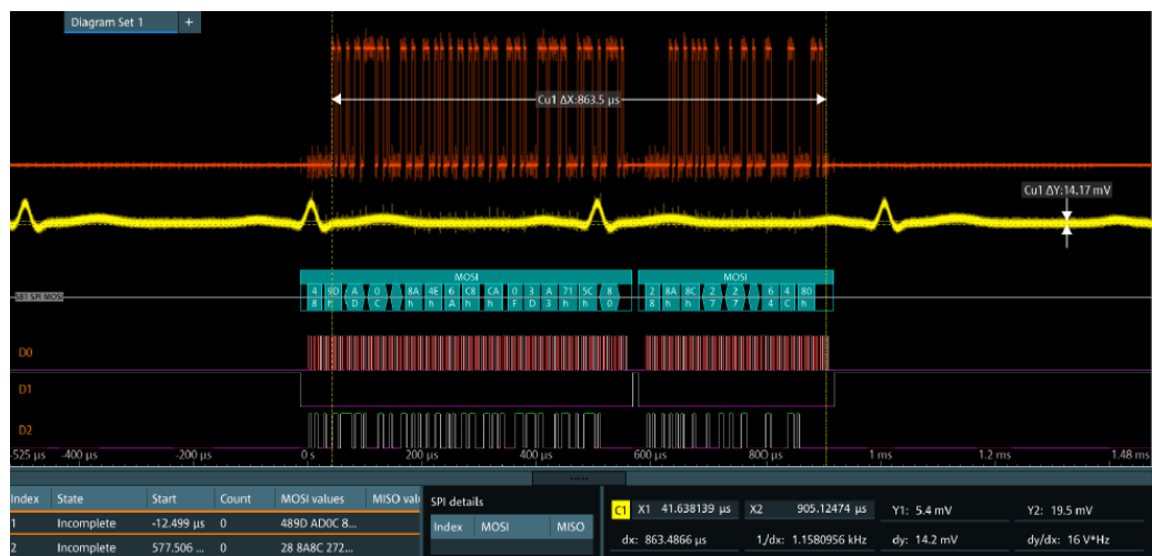
Figure 13-3: Decoded and binary SPI signal
