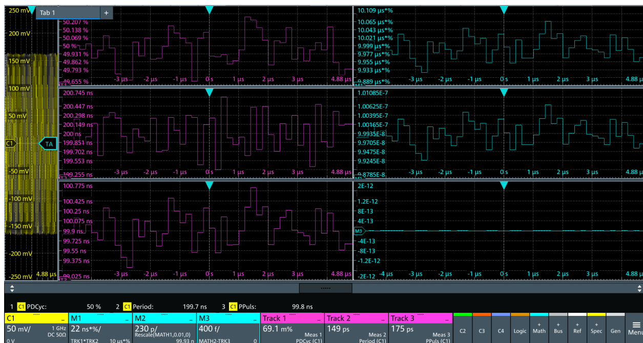
Figure 9-7: Tracks used in math functions
