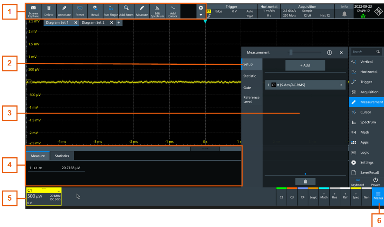
Figure 4-6: Control elements on the graphical user interface
