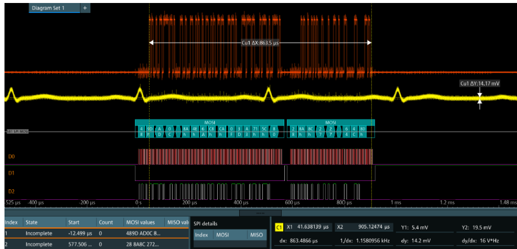
Figure 13-3: Decoded and binary SPI signal
