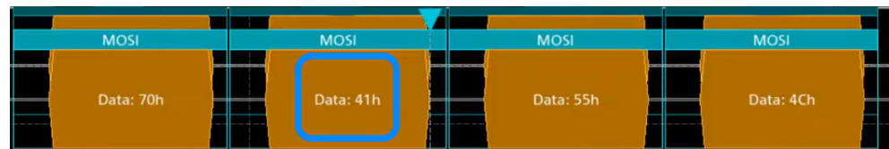
Figure 13-4: Trigger on Type= MOSI, Data pattern = 41
