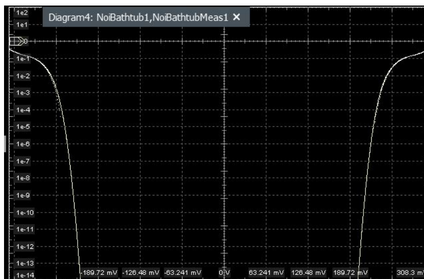
Figure 19-16: Bathtub plot for NRZ signals
