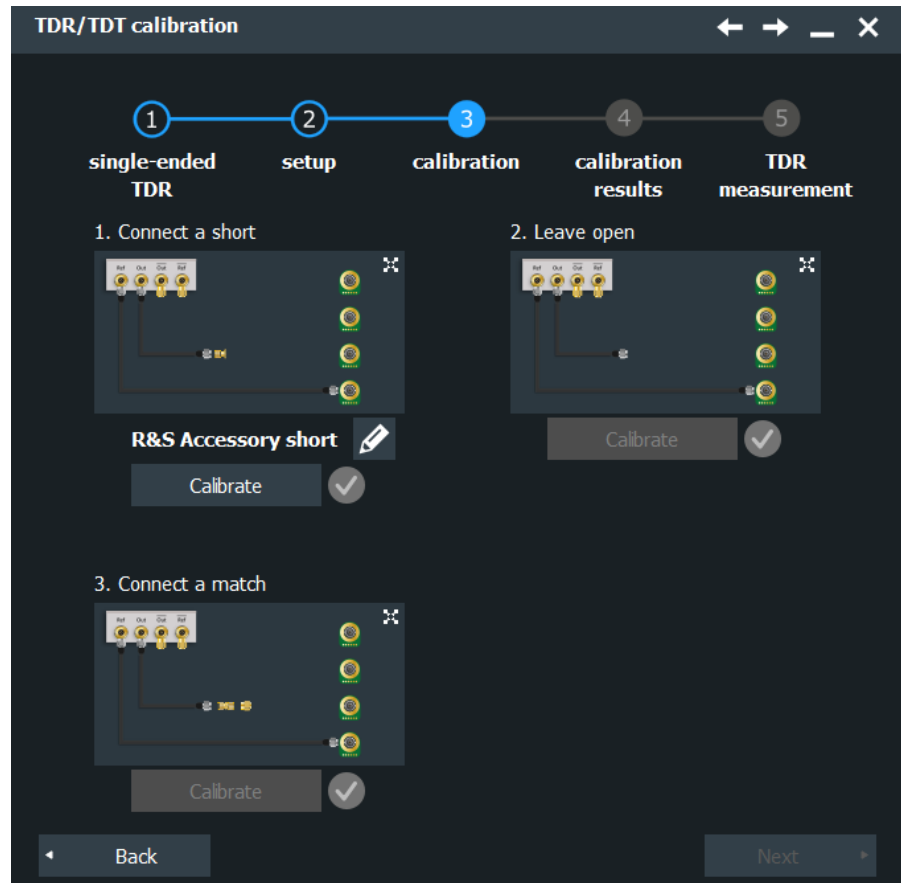
Figure 17-3: Calibration of single-ended TDR/TDT
