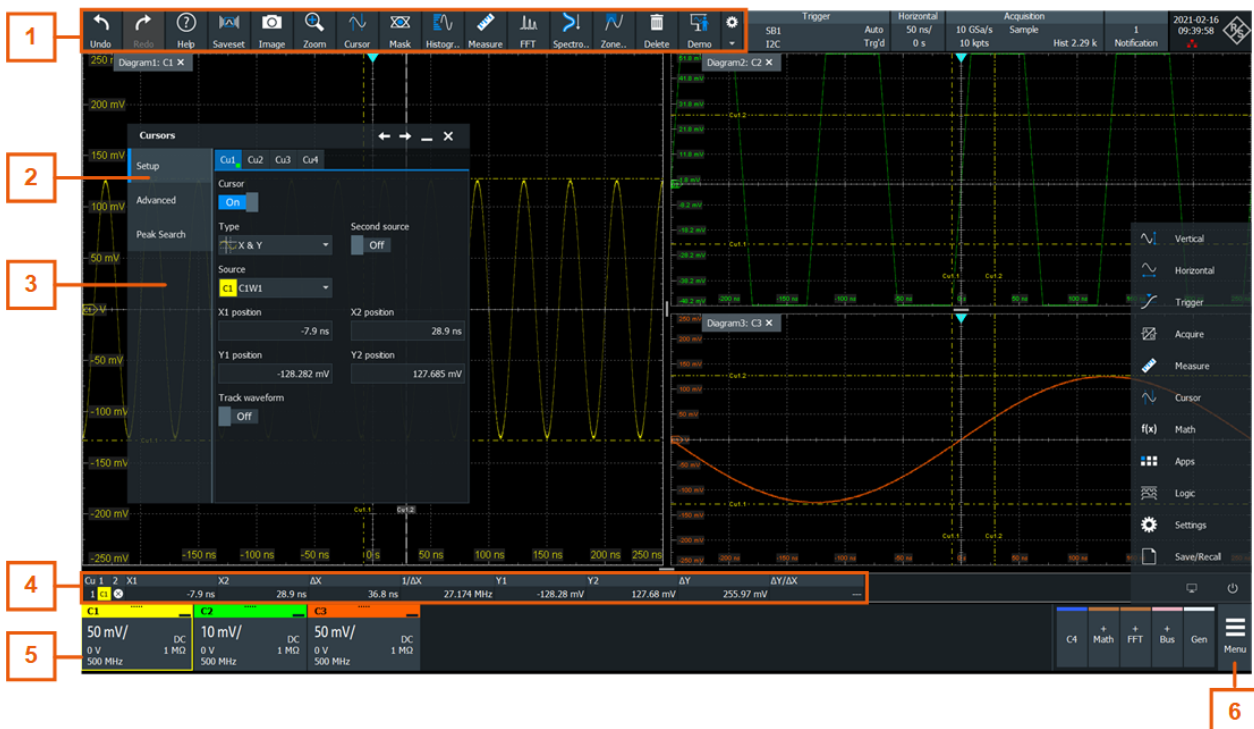
Figure 3-8: Control elements on the touchscreen
