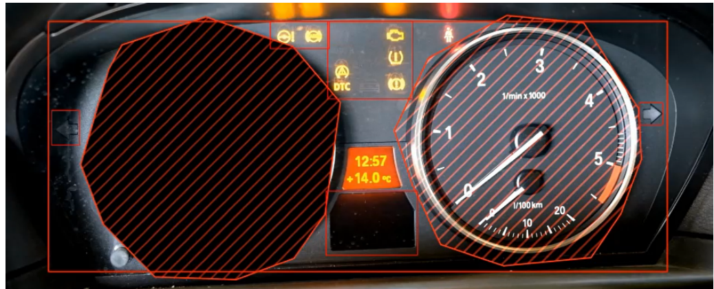
Figure 5-31: Example of a recording with two Ignore Area polygons
