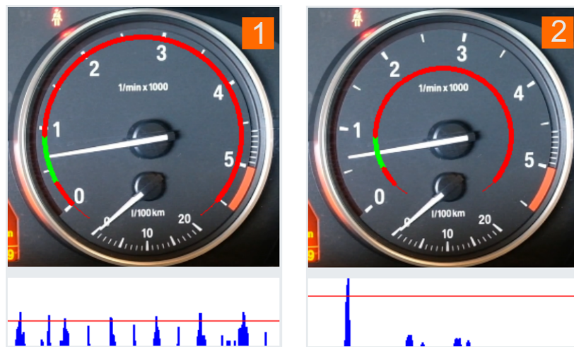
Figure 6-23: Bad and good choice for the radius of an indicator detection line
