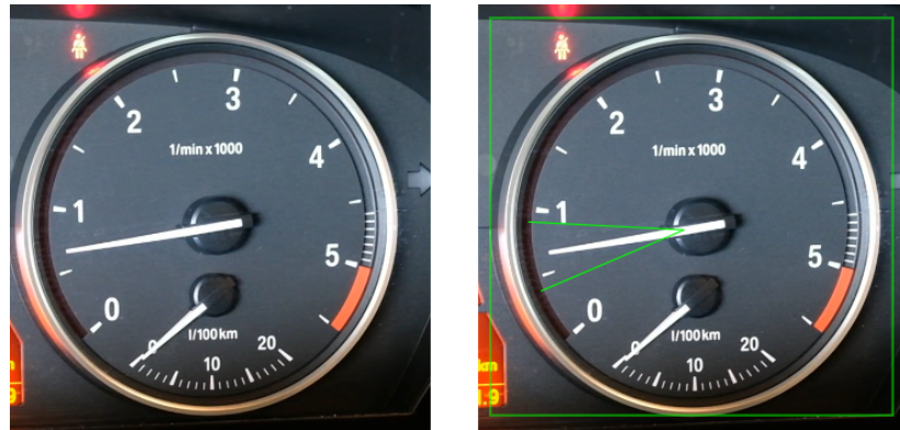
Figure 6-21: Configured needle-type pointer
