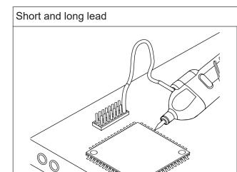
The lead provides a flexible connection to the DUT. It is plugged onto a pin on the DUT and can be used to connect either the signal socket or the ground socket. In addition, it allows micro and mini clips to be connected to the probe.
