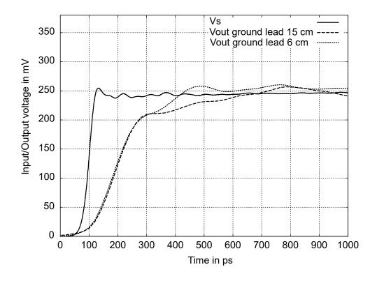
Figure 4-7: Step response of the R&S RT-ZS30 with a type 2 connection
