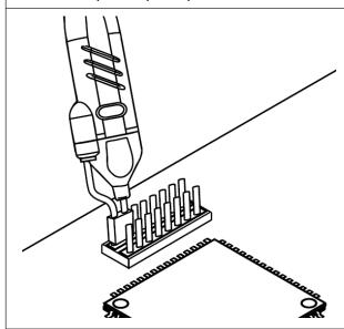
The ground adapter is used for plugging the probe onto pin strips with 0.64 mm square pins (typical pitch 2.54 mm, 100 mil).
