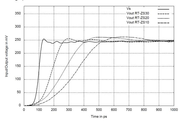
Figure 4-4: Step response of the R&S RT-ZS10/20/30
