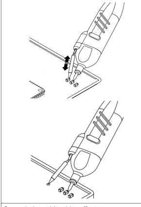
The spring-loaded ground pin allows handheld probing. Because this ground pin compensates for minor unevenness and movements, it can establish a firm contact with the test point. It fits into the ground socket of the probe head.
