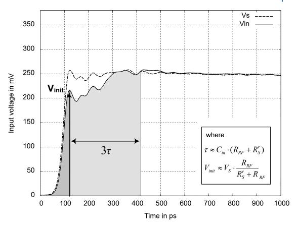
Figure 4-10: Signal loading caused by the R&S RT-ZS10/20/30 probe at an effective source impedance of 25  $\Omega$
