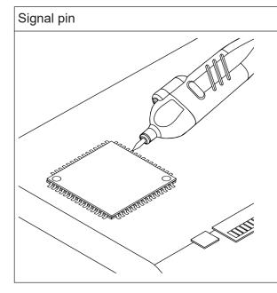
The signal pin is held to the DUT to tap off the measurement signal. It fits into the signal socket and is designed for various applications, e.g. measurements on SMT resistors, IC pins, conductors or vias.
