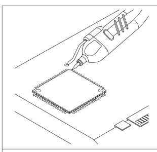
The rigid ground pin is soldered to a test point on the DUT and provides a reliable and permanent connection to the DUT.
