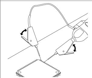
The micro clip is designed for probing IC pins and thin wires in fine-pitch applications.
