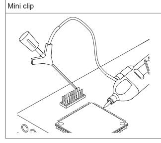
The mini clip is designed for probing large IC pins, wires and through-hole components.
