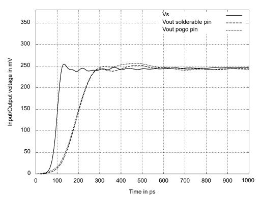
Figure 4-6: Step response of the R&S RT-ZS30 with a type 1 connection
