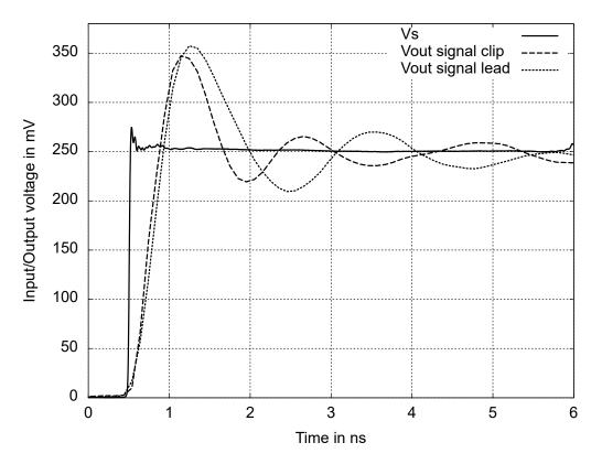
Figure 4-8: Step response of the R&S RT-ZS30 with a type 3 connection
