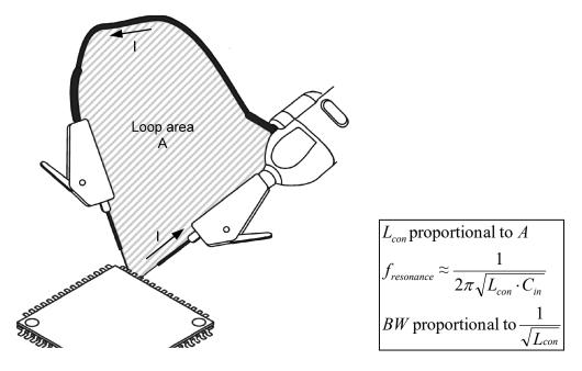
Figure 4-5: Ground connection and connection inductance
