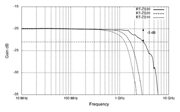
Figure 4-3: Amplitude/frequency response of the R&S RT-ZS10/20/30
