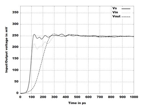
Figure 4-11: Unloaded and loaded input signal and step response (for RT-ZS30)
