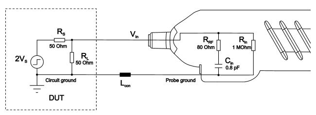
Figure 4-2: Equivalent circuit model of the R&S RT-ZS10/20/30 probe
