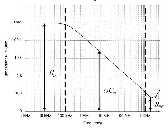
Figure 4-9: Magnitude of the input impedance of the R&S RT-ZS10/20/30 probe as a function of frequency
