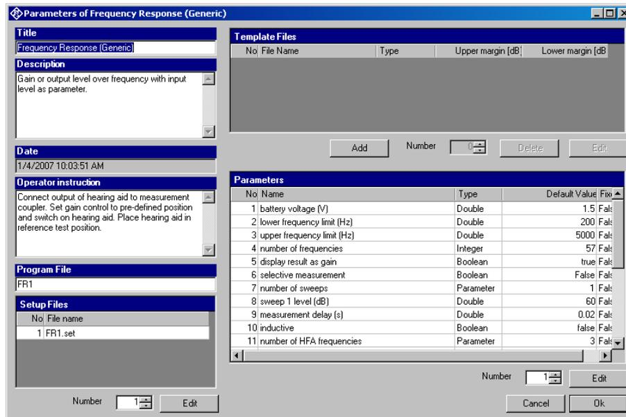
Figure 6-6 Measurement setup window
