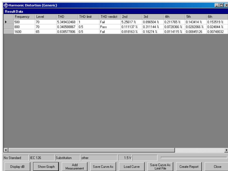
Figure 6-15 Data table display of harmonic distortion measurement
