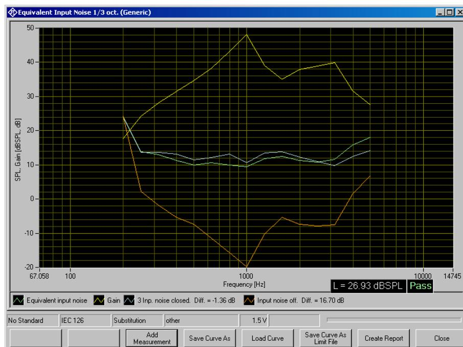
Figure 6-21 Measurement window for equivalent input noise
