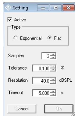
Figure 3-3 Input window for adaptive measurement
