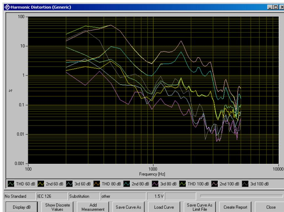
**Figure 6-14** Curve display of harmonic distortion measurement
