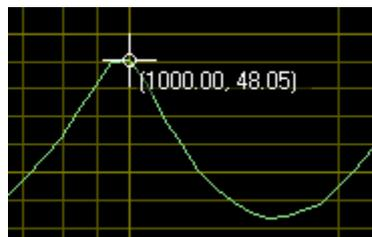
Figure 6-4 Cursor with data display
