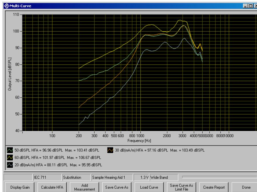
Figure 6-11 Display window of multi-curve measurement
