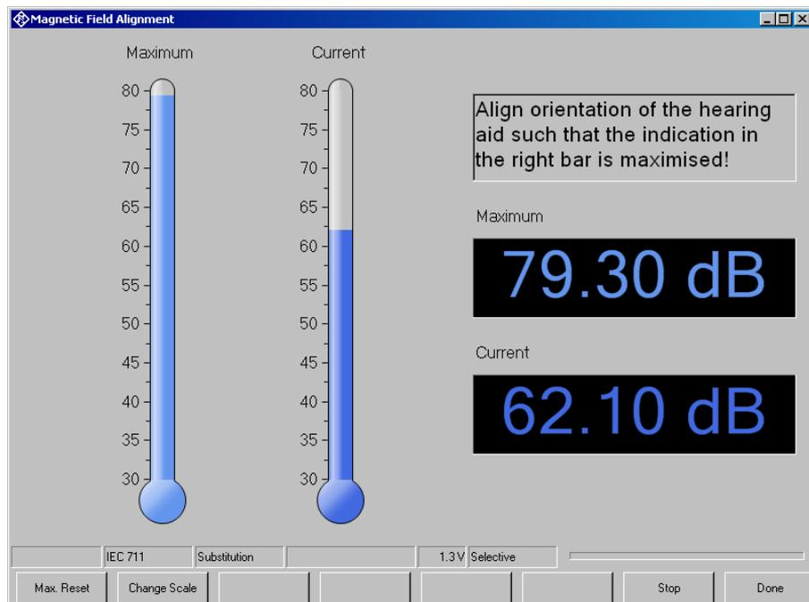
Figure 6-28 Display of the routine for magnetic field alignment
