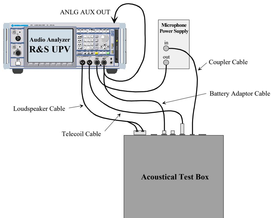
Figure 2-1 Test setup and connection of external components
