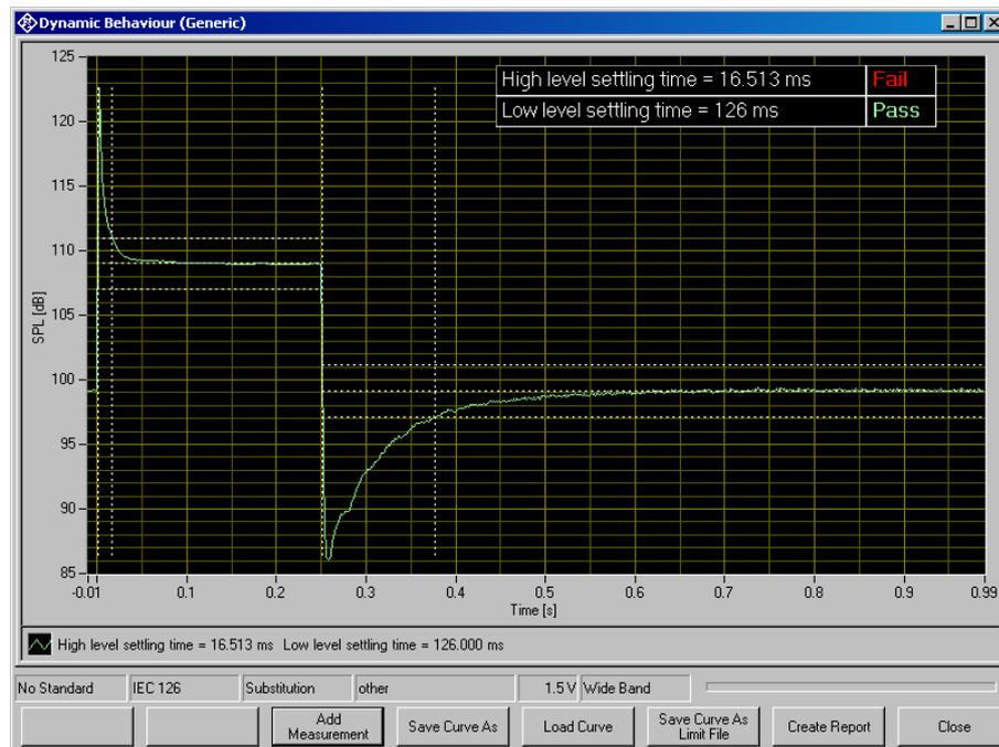
**Figure 6-18 Measurement window for dynamic behaviour**
