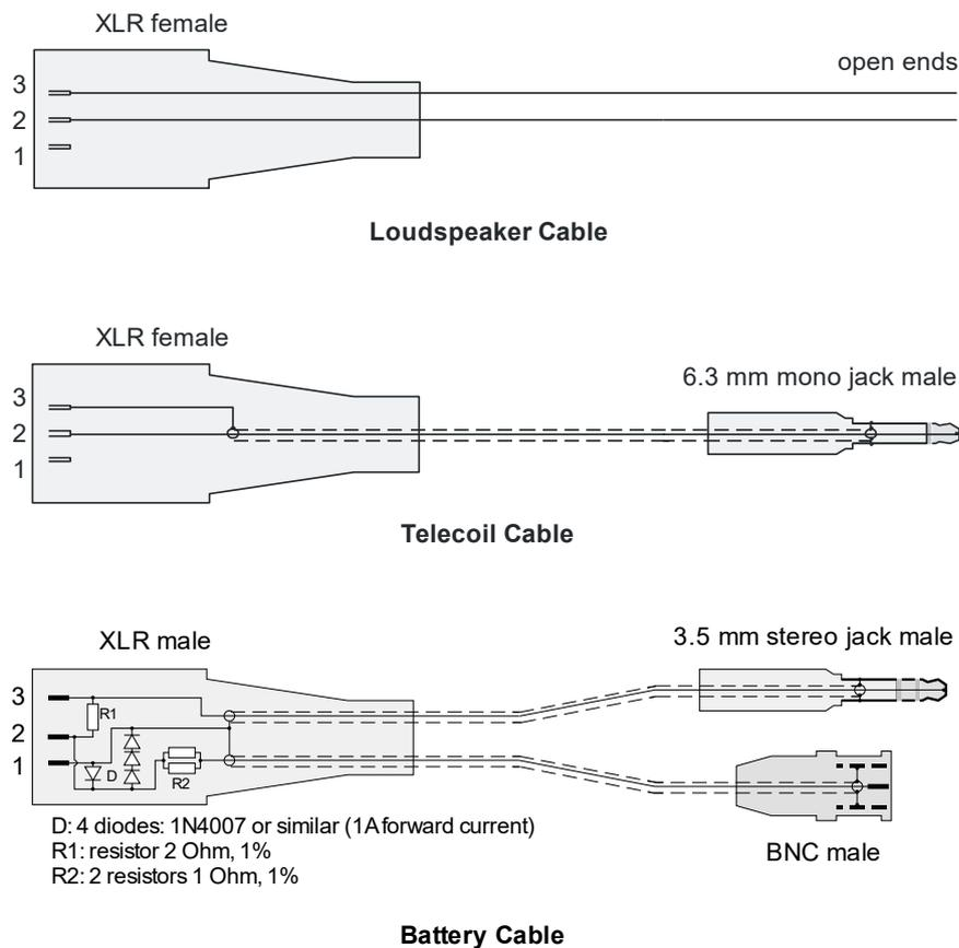
Figure 2-2 Connection cables for R&S UPL-B7 (Interacoustics TBS 25) test box
