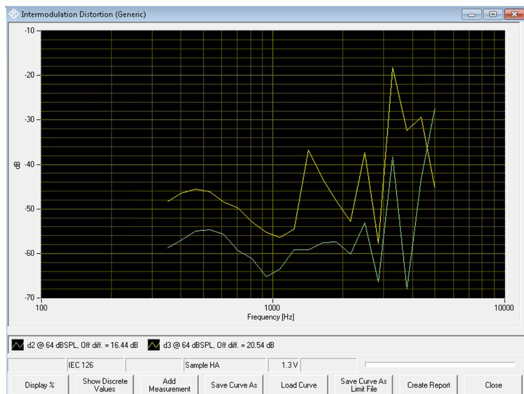
**Figure 6-16** Curve display of intermodulation distortion measurement
