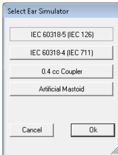
Figure 2-5 Query window for selection of ear simulator
