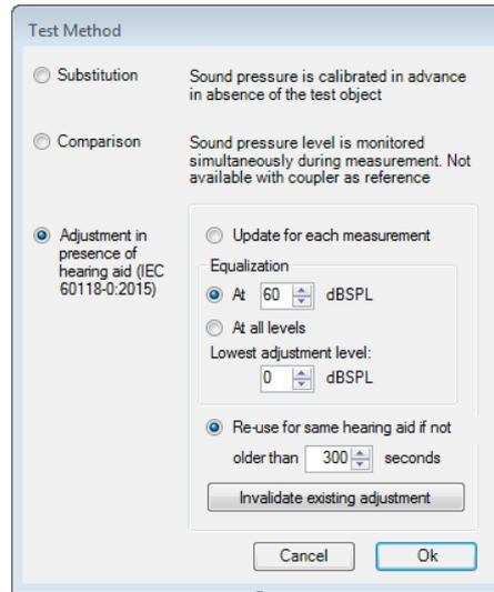
**Figure 3-4: Window for selection of the test method**
