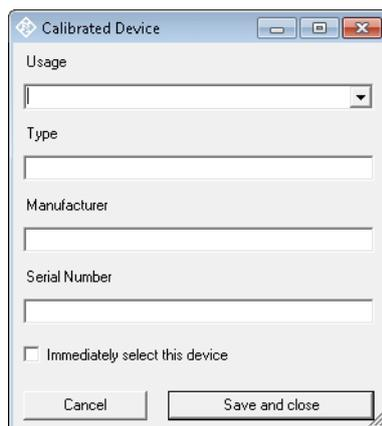
Figure 4-2 Input window for information about calibrated device
