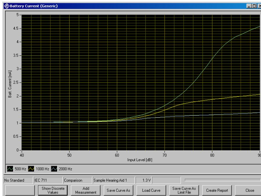
Figure 6-22 Graphic display of battery current measurement
