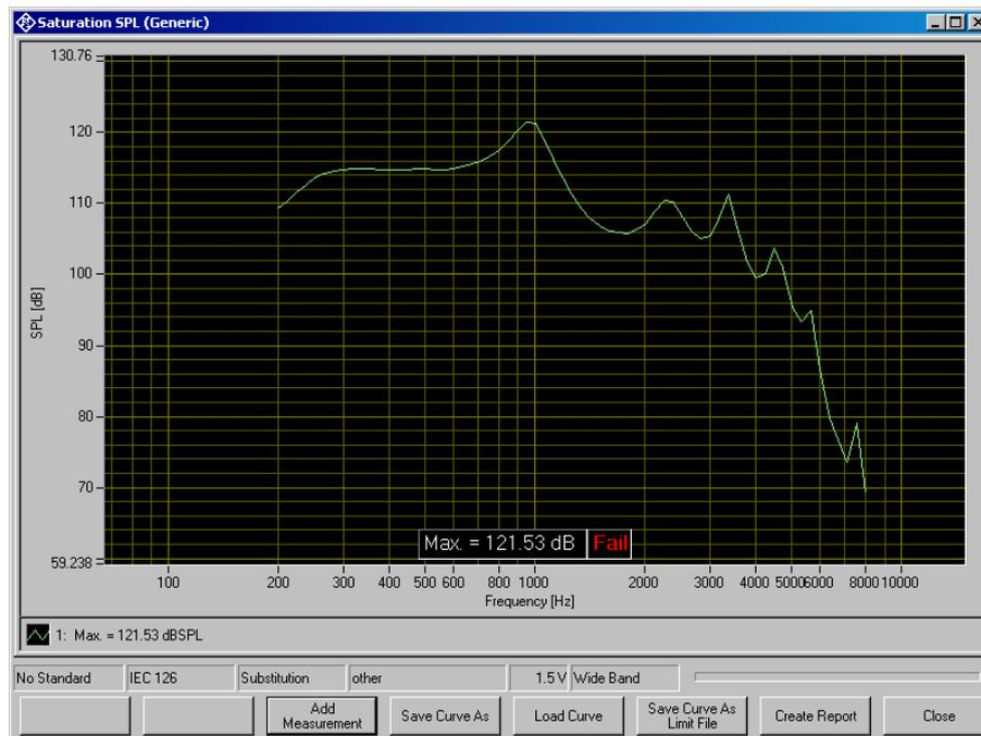
**Figure 6-13** Display window of saturation sound pressure level measurement
