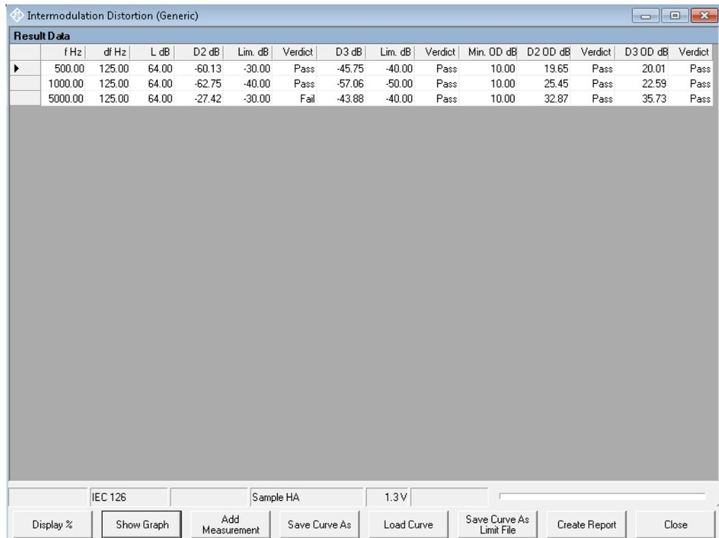
Figure 6-17 Data table display of intermodulation distortion measurement
