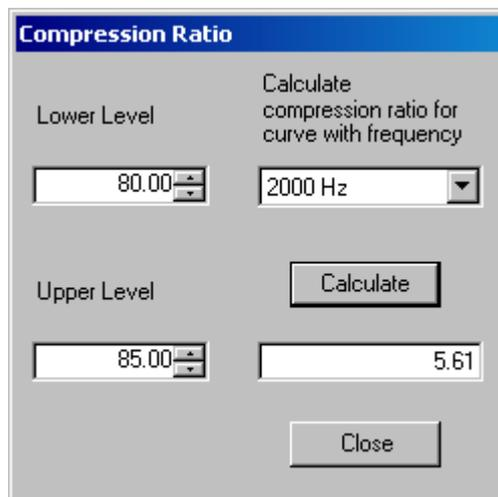
**Figure 6-20 Window for calculation of compression ratio**
