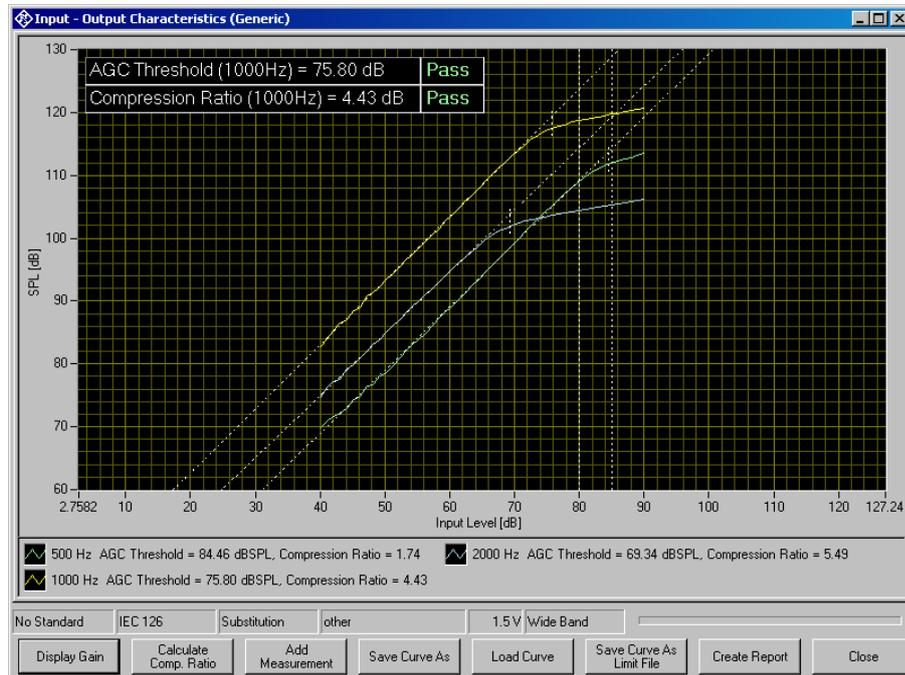
**Figure 6-19 Measurement window for input-output characteristics**
