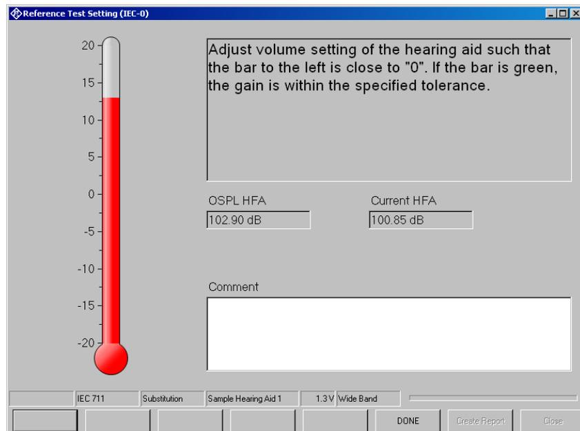
**Figure 6-26** Initial display of the routine for reference test gain setting
