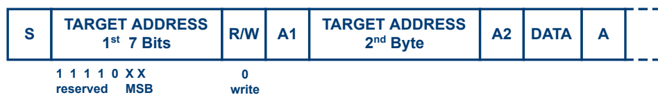
Figure 14-2: 10-bit address, write access
