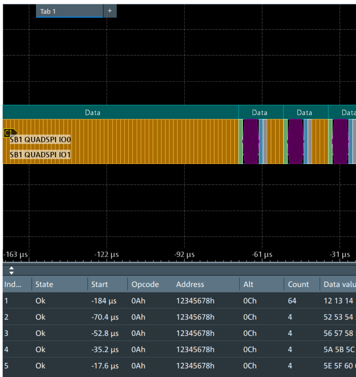
Figure 13-5: Decoded QUAD-SPI signal
