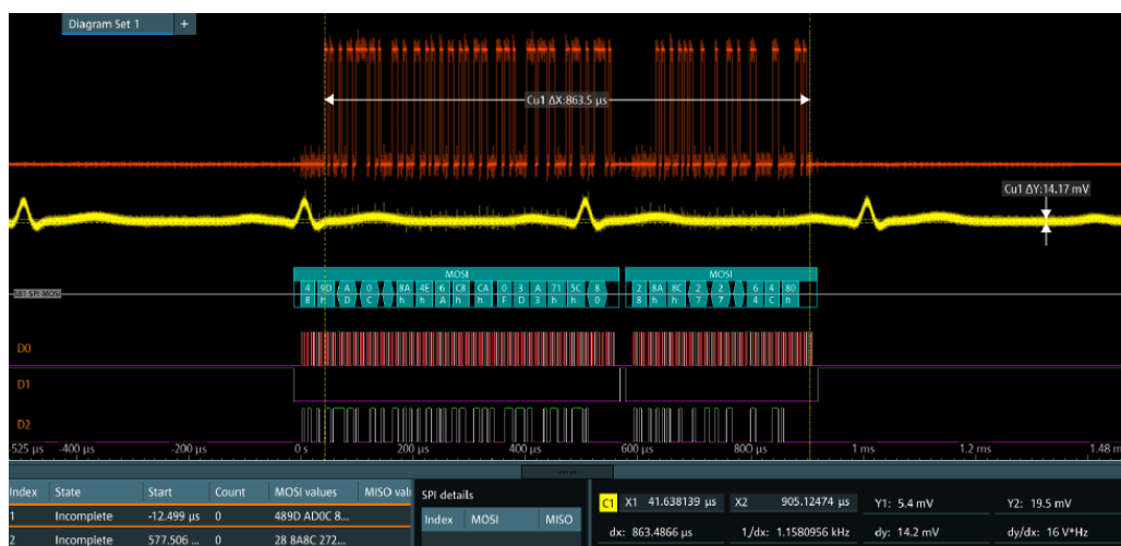
Figure 13-3: Decoded and binary SPI signal
