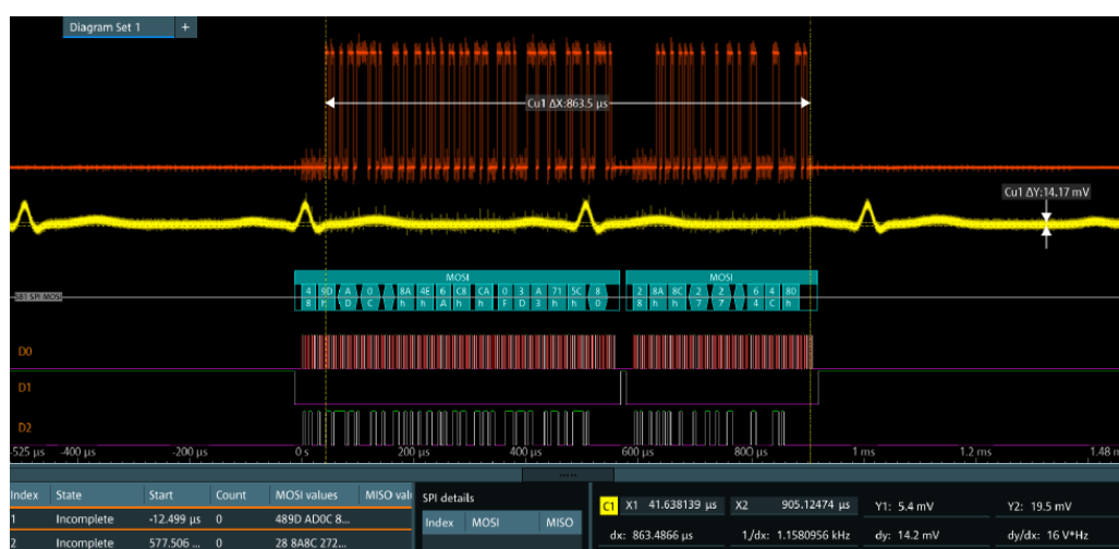
Figure 13-3: Decoded and binary SPI signal
