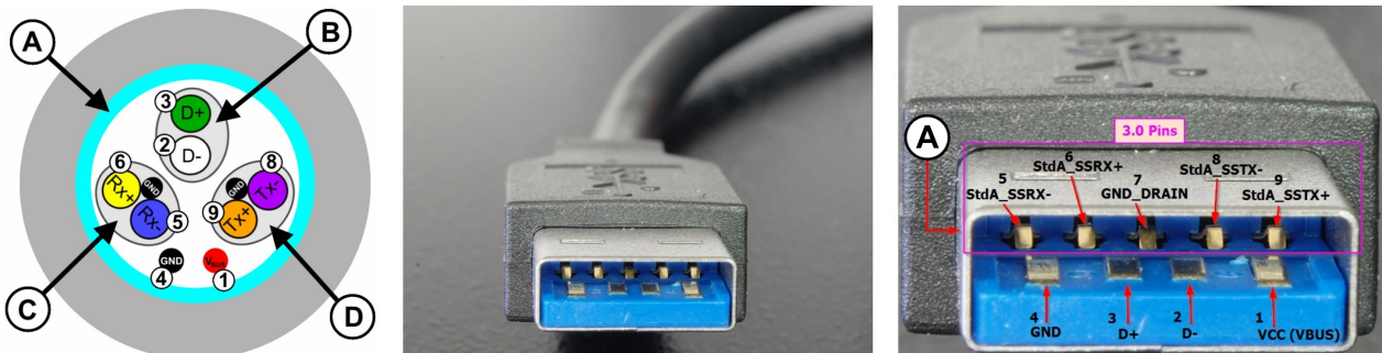
Figure 14-38: USB 3.1 cable cross-section and Standard-A plug - backward compatible with USB 2.0
