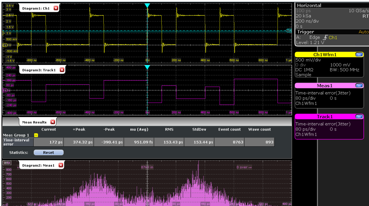
Figure 19-3: TIE measurement with CDR trigger, 10 Mbps, with track and histogram
