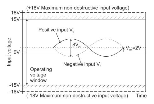
Figure 4-2: Voltage operating window
