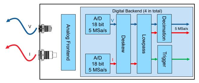
Figure 4-3: Signal flow with an oscilloscope
