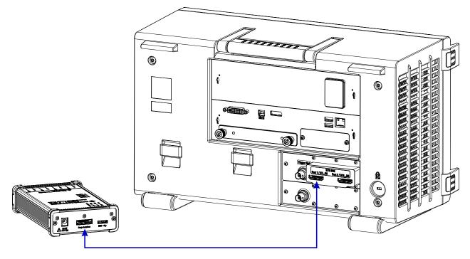
Figure 3-1: Connecting the probe to the oscilloscope
