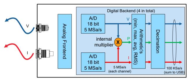
Figure 4-4: Signal flow with R&S CMWrun
