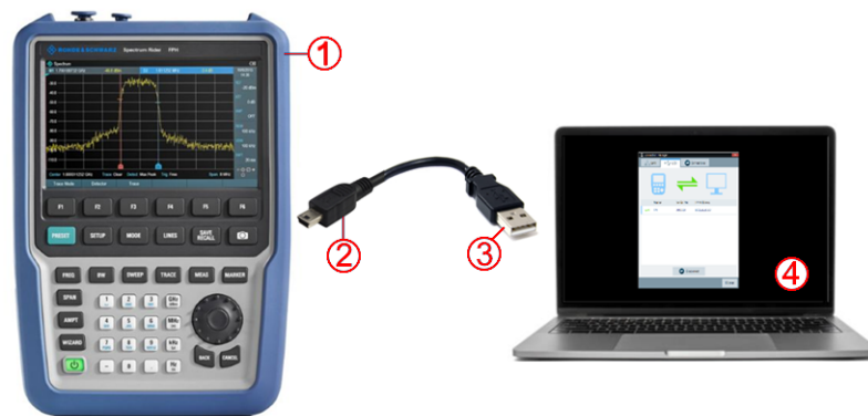
Figure 2-3: Connecting R&S FPH to a laptop with a USB cable
