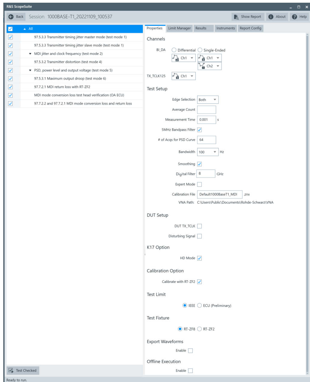
Figure 9-1: Configuration for 1000BASE-T1 compliance tests
