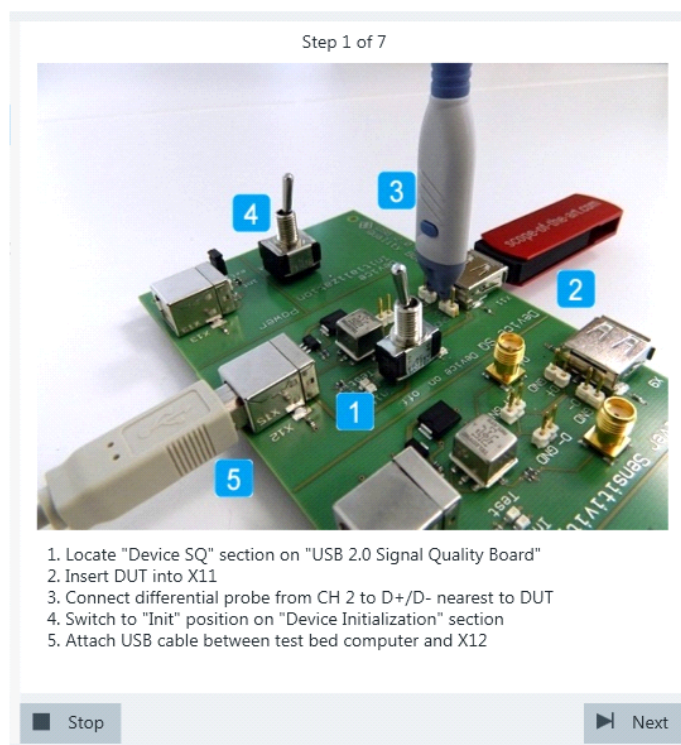
Figure 4-1: R&S RT-ZF1: connection to DUT
