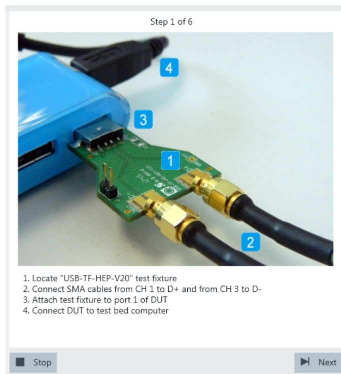
Figure 4-10: USB-IF USB2.0 hi-speed signal quality host test fixture: connection to DUT
