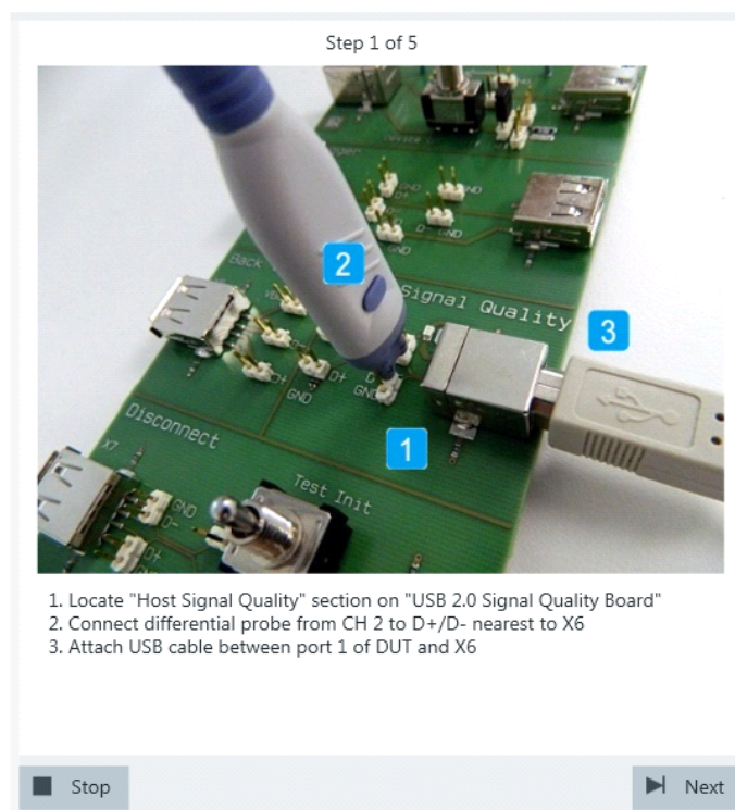
Figure 4-11: R&S RT-ZF1: connection to DUT
