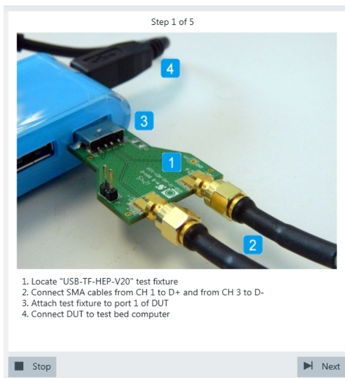
Figure 4-8: USB-IF USB2.0 Hi-Speed Signal Quality host test fixture: connection to DUT
