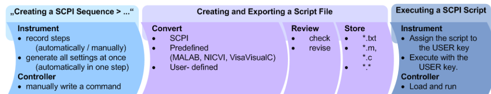
Figure 12-7: Steps for performing SCPI Scripts
