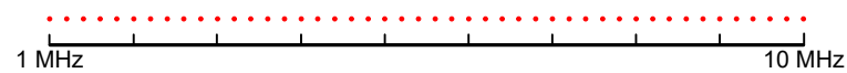
Figure 4-1: Linear x-axis scaling: the distance between the measurement points is equal, e.g. 200 kHz
