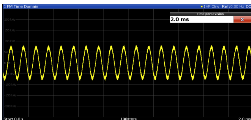
Figure 3-3: FM time domain measurement with time domain zoom (2.0 ms per division)
