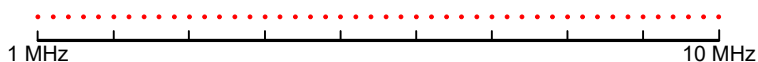
Figure 4-2: Linear x-axis scaling: the distance between the sweep points is equal, e.g. 200 kHz
