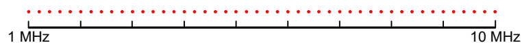
Figure 10-3: Linear x-axis scaling: the distance between the measurement points is equal, e.g. 200 kHz
