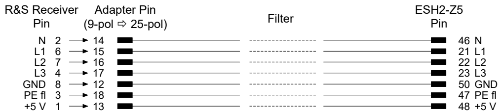
Figure 9-3: Connection from R&S EPL1000 to R&S ESH2-Z5
