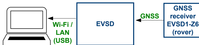
Figure 8-2: Configuring the R&S EVSD1-Z6 GNSS RTK device (rover) via the R&S EVSD1000
