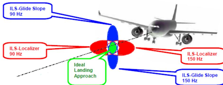
Figure 3-2: Approach navigation using instrument landing system (ILS)
