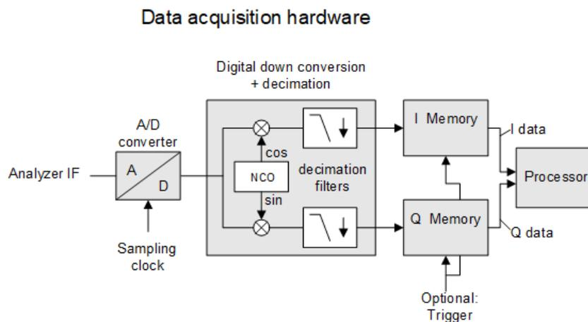
Figure 3-8: Block diagram of analyzer signal processing
