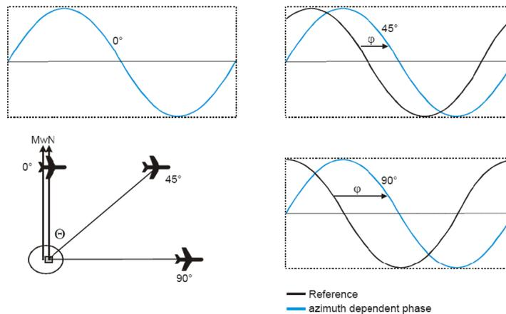
**Figure 3-3: Basics of the VOR phase angles ( $\Phi$ ) depending on the azimuth angle ( $\Theta$ )**
