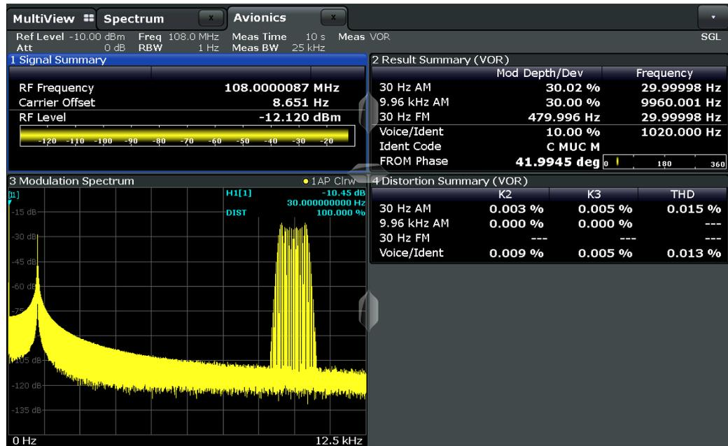
Figure 9-3: Results of the remote VOR measurement
