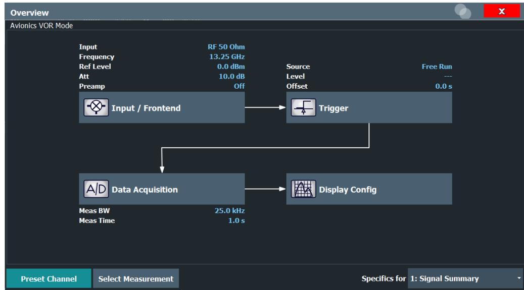
In addition to the main measurement settings, the "Overview" provides quick access to the main settings dialog boxes. The individual configuration steps are displayed in the order of the data flow. Thus, you can easily configure an entire measurement channel from input over processing to output and analysis by stepping through the dialog boxes as indicated in the "Overview".
