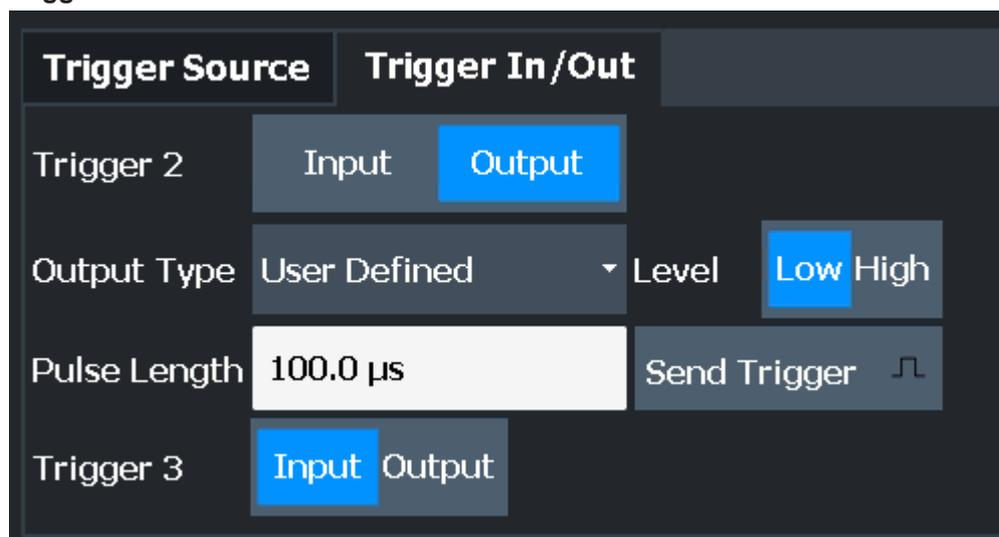
The trigger input and output functionality depends on how the variable "Trigger Input/Output" connectors are used.
