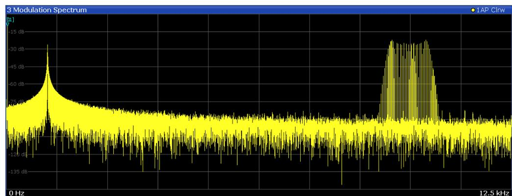
Figure 4-6: Modulation spectrum for a VOR signal
