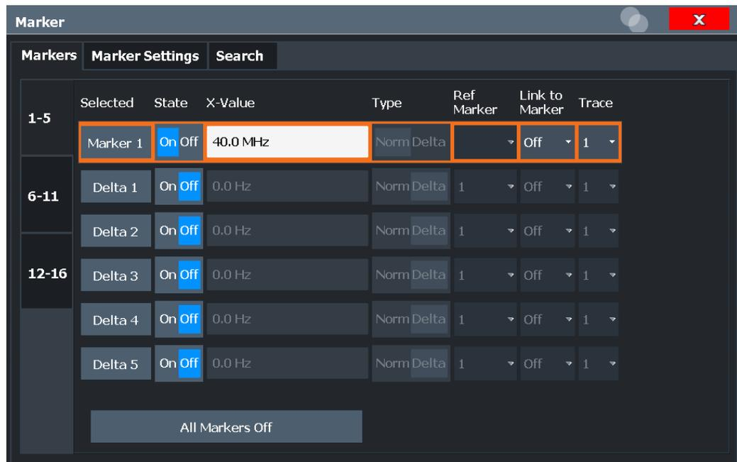
The markers are distributed among three tabs for a better overview. By default, the first marker is defined as a normal marker, whereas all others are defined as delta markers with reference to the first marker. All markers are assigned to trace 1, but only the first marker is active.
