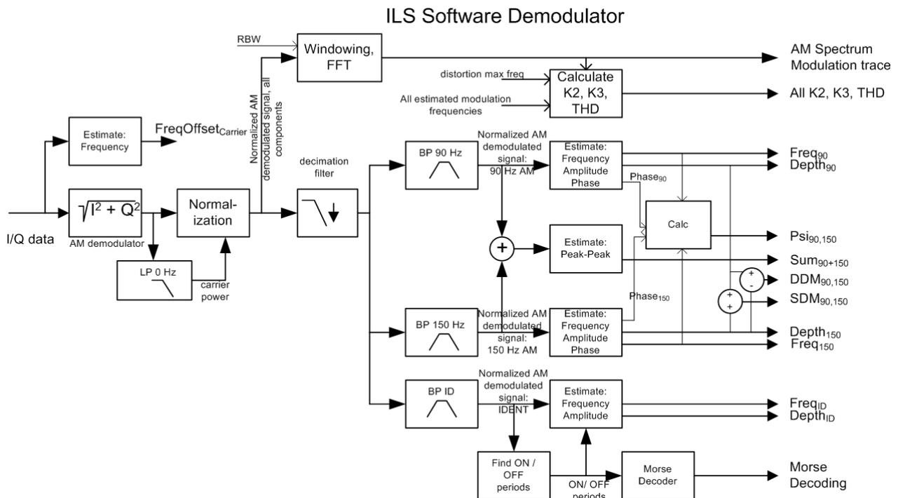
Figure 3-9: Block diagram of ILS software demodulator
