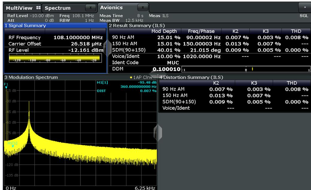
Figure 9-2: Results of the remote ILS measurement
