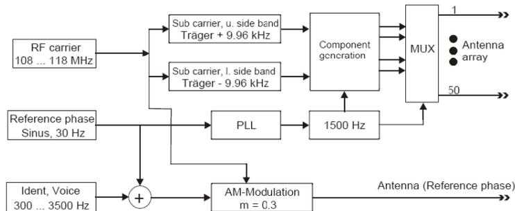
Figure 3-7: Basics of the DVOR signal generation
