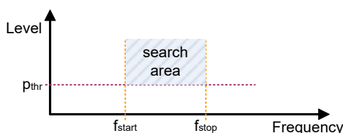
Figure 6-2: Basic principle of the signal search feature
