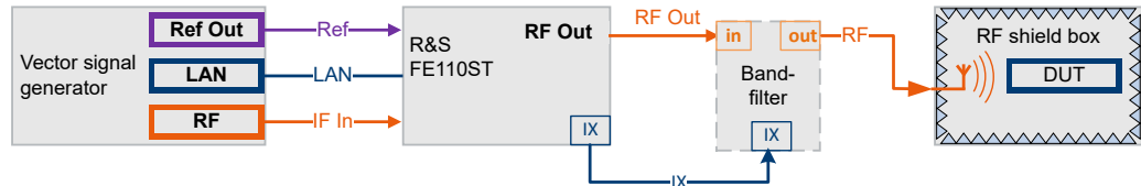
Figure 3-10: Test setup: Vector signal generator with R&S FE110ST and external device
