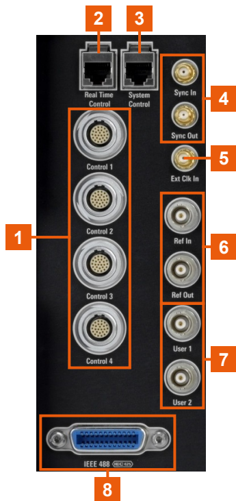
Figure 3-5: Connectors for control, synchronization and multi-purpose signals
