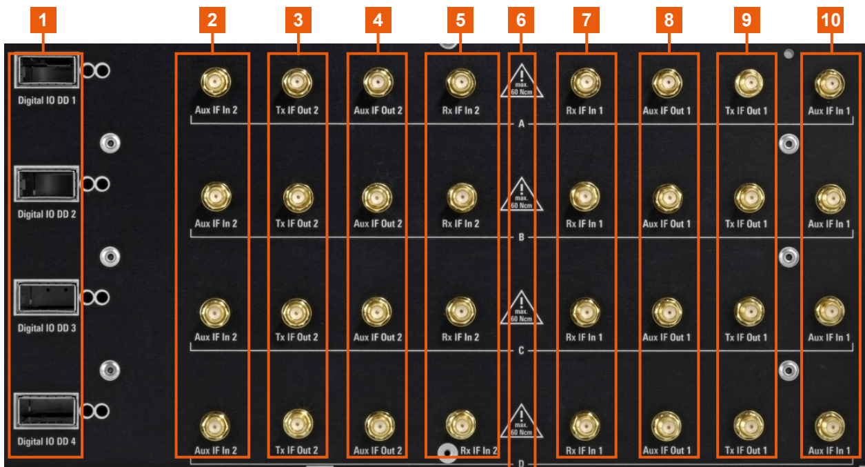
Figure 3-7: Digital IO DD connectors and instrument boards
