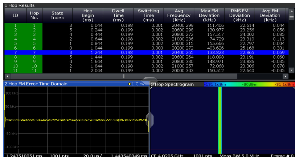
Figure 8-4: Effect of the FM video bandwidth
