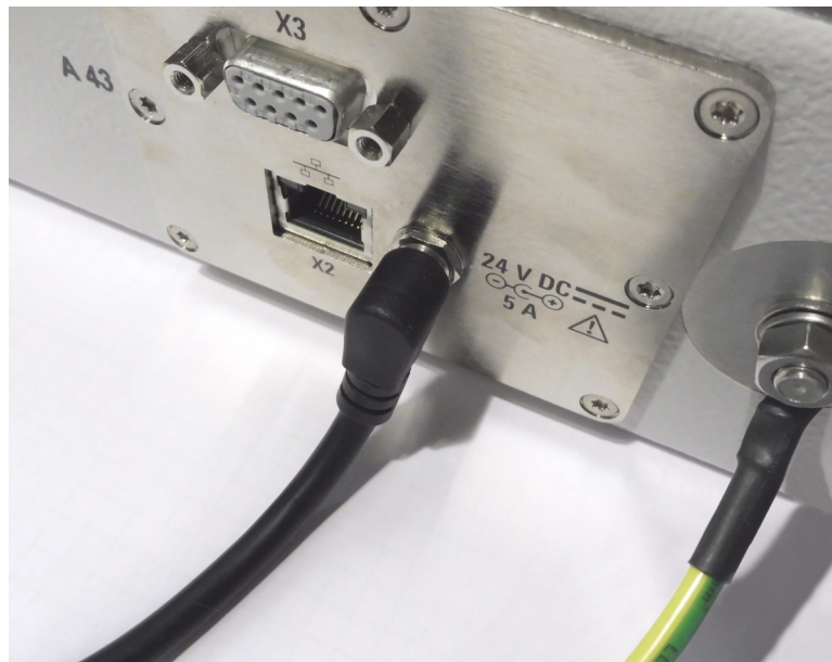
Figure 7-1: 24 V DC power supply connector [X1] (center)
