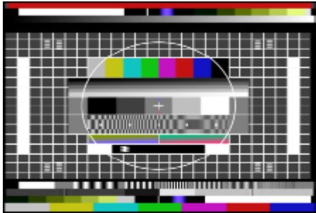
Figure 2-1: Codec 4:3 test pattern
