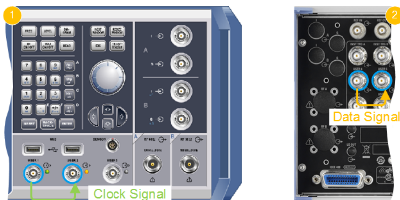
Figure 2-6: Looping back of the clock and data signals (the BER Data Enable signal is routed internally)
