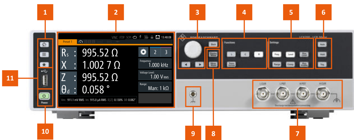
Figure 4-4: R&S LCX front panel
