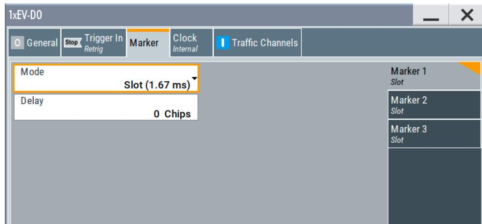
The dialog provides settings to select and configure the marker output signal including marker mode and marker delay.
