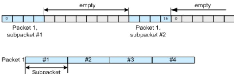
Only one configurable packet is available for physical layer subtype 0&1, the data channel is continuously active for the number of packets to send.
