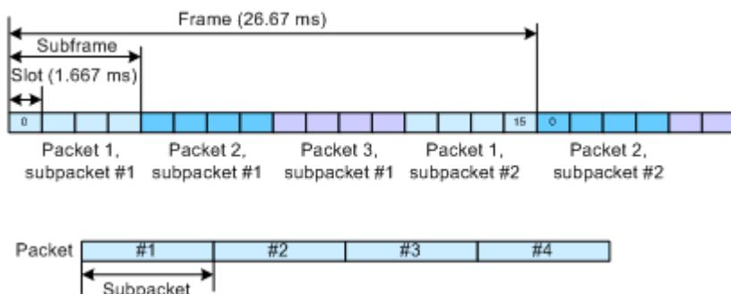
When only one packet is active and "Number of Subpackets" is set to 1, no interleaving is performed between the packets. In this case, the data channel is active continuously (see figure below).
