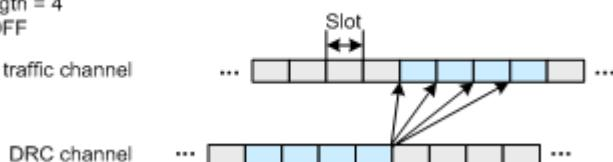
If gating is active, each value of the DRC channel is transmitted for one slot followed by DRCLenght-1 empty slots.
