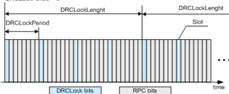
**Note:** A value of zero disables the DRC lock subchannel and the MAC RPC channel of the selected user is not punctured with the DRC lock subchannel.
