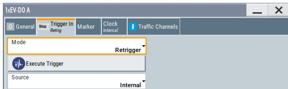
This tab provides settings to select and configure the trigger, like trigger source, trigger mode and trigger delays, and to arm or trigger an internal trigger manually. The header of the tab displays the status of the trigger signal and trigger mode. As in the tabs "Marker" and "Clock", this tab provides also access to the settings of the related connectors.
