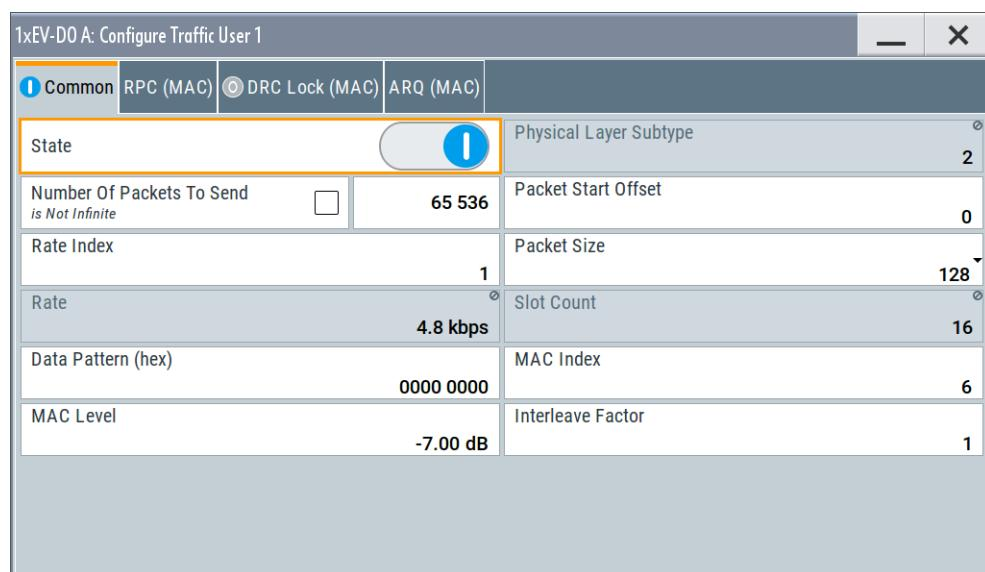
The dialog comprises the settings of the traffic channel and of the forward MAC channel settings, such as Reverse Power Control (RPC) and DRCLock.
