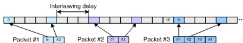
**Note:** An offset value of zero with a rate change from a single slot packet to multiple slot packets causes the first slot of the multiple slot packets to be transmitted in the slot immediately following the single slot packet.
