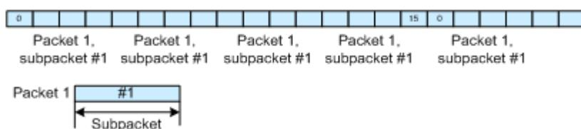
When only one packet is active but the number of subpackets is larger than one, interleave subframe. In this case, two subframes are left empty in-between every two subpackets (see figure below).
