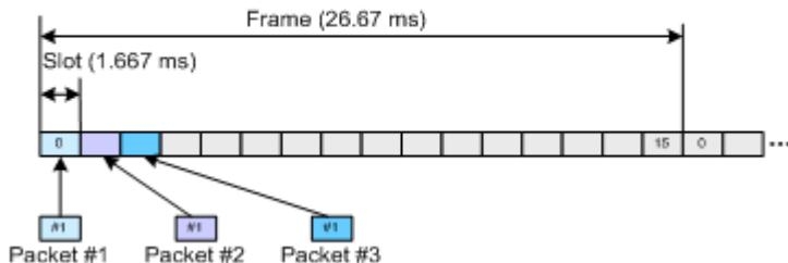
For multiple slot packets, a value of zero will cause the next packet transmission to start three slots after the end of the previous packet. The three slot delay is identical to the interleaving delay between slots for multiple slot packets. The offset value is attached to the end of the preceding packet.
