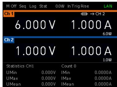
Figure 5-7: Linking of channel 2 to channel 1
