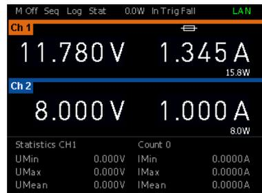
Figure 5-6: Fuse indicator display at channel 1
