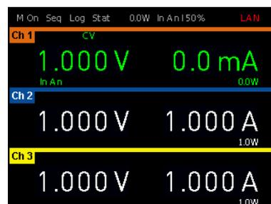
Figure 5-11: Analog In example for R&S NGC103(-G)
