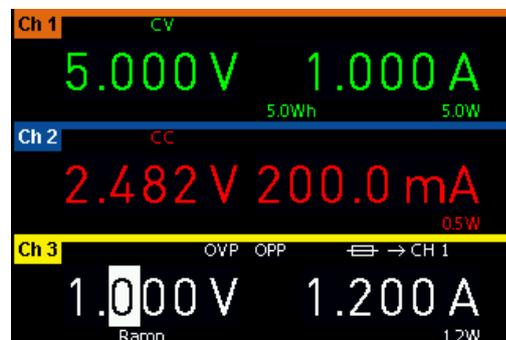
Figure 3-11: Color coding of difference operating conditions
