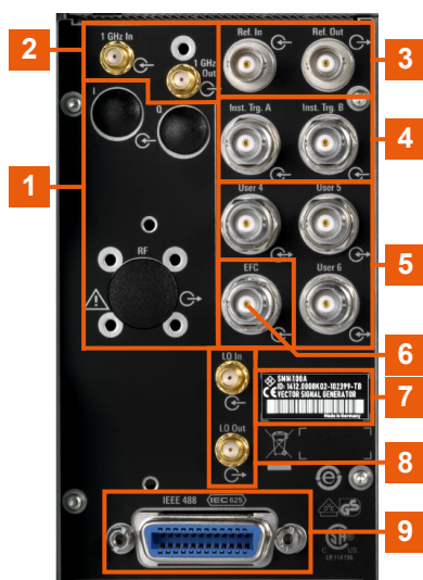
Figure 3-5: Connectors for multipurpose RF signals and remote control
