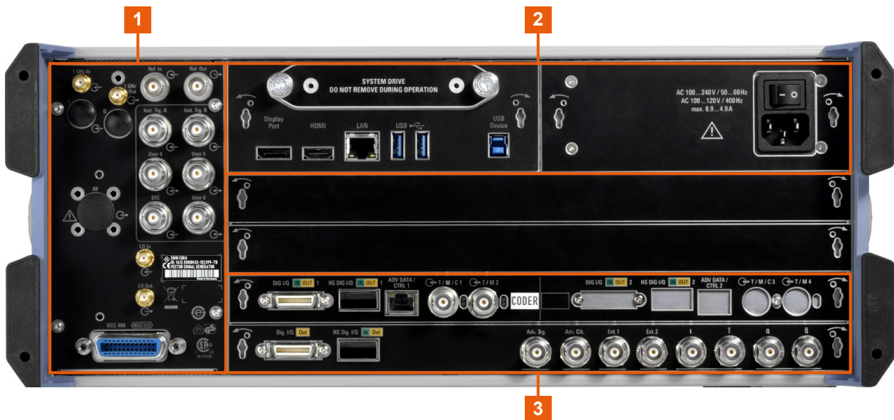
Figure 3-4: R&S SMM100A rear panel connectors
