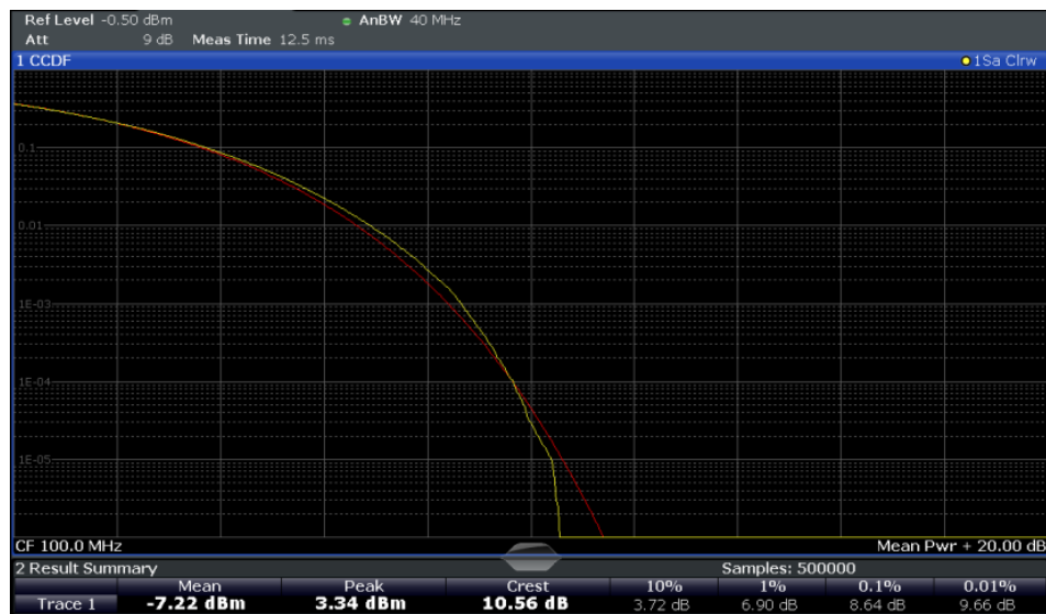
Figure 3-34: CCDF measurement results
