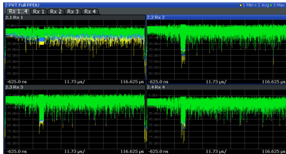
Figure 3-21: PvT Full PPDU result display for IEEE 802.11n MIMO measurements
