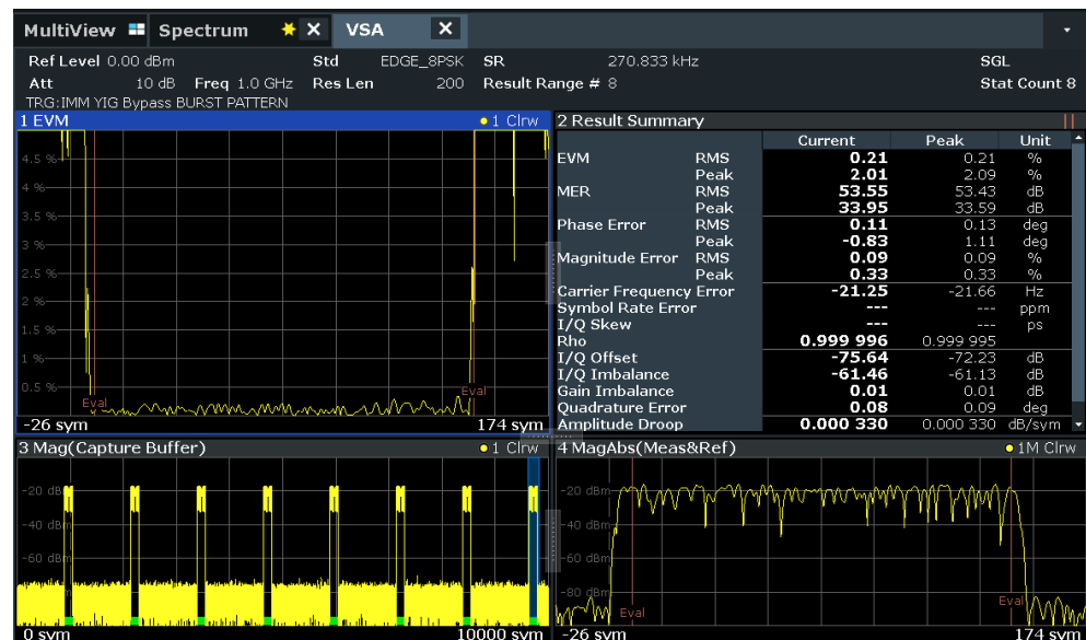
Figure 8-8: Result range that exceeds the burst length
