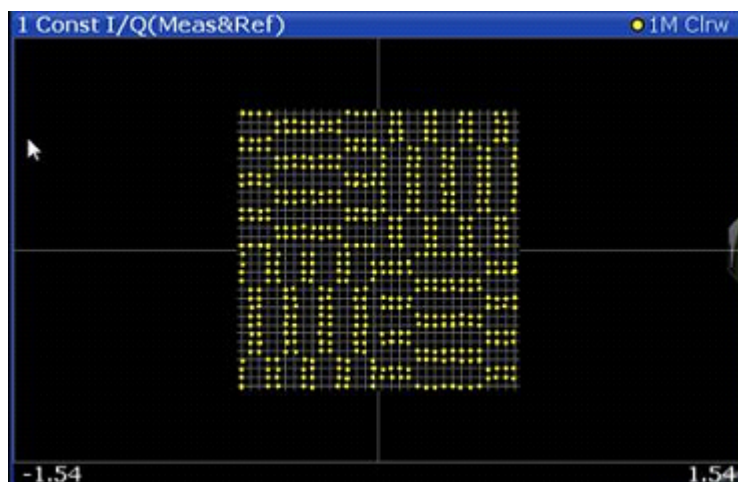
Figure 9-12: Constellation diagram for 1024QAM modulation and PRBS9
