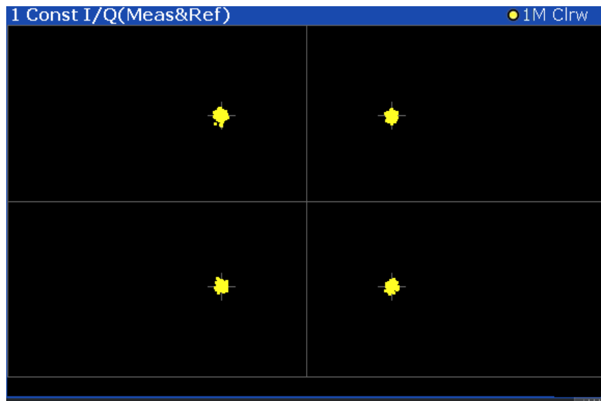
Figure 3-3: Constellation I/Q diagram for QPSK modulated signal
