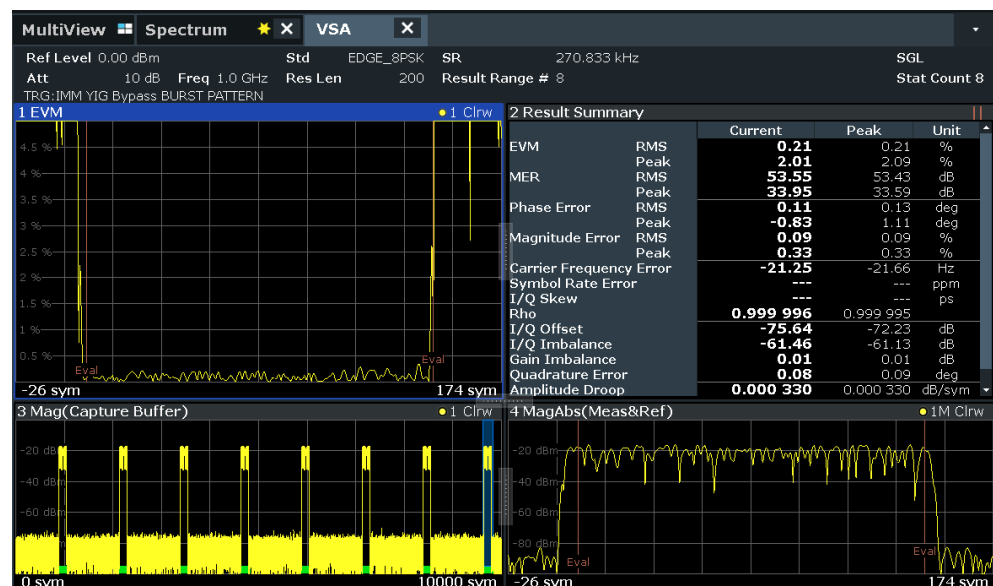
Figure 9-8: Result range that exceeds the burst length
