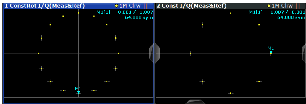
Figure 3-5: Constellation I/Q (Rotated) result display vs. common Constellation I/Q for 3\pi/8 -8PSK modulation
