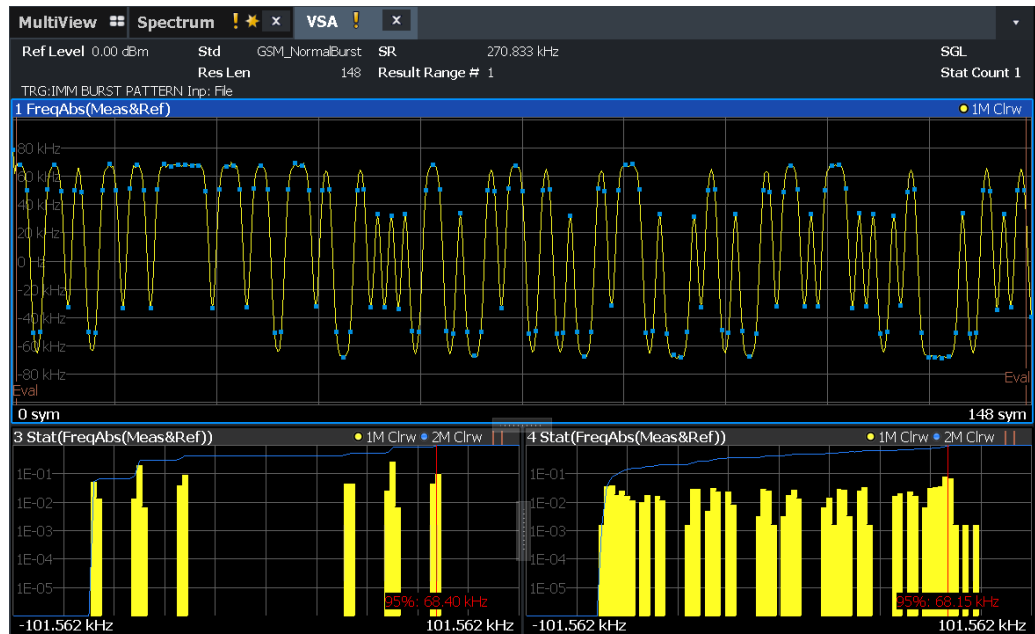
Figure 6-2: Statistics measurement: window 1: measured signal (symbols highlighted); window 3: statistics for symbol instants only; window 4: statistics for all trace points;
