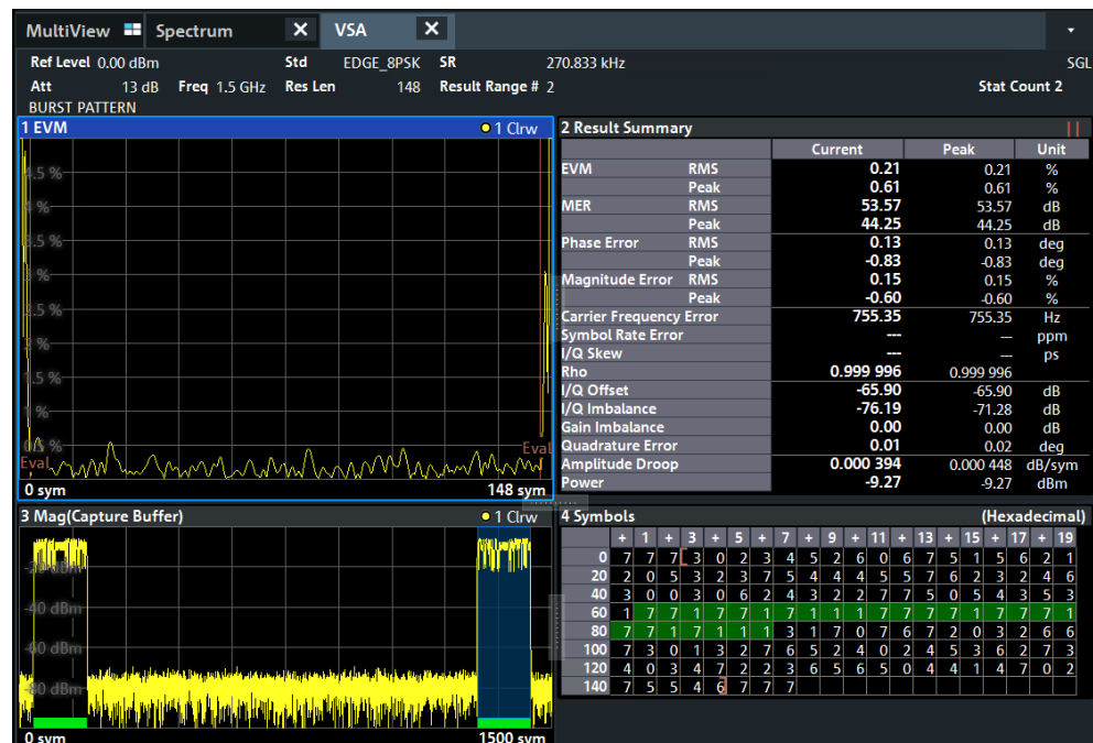
Figure 9-6: Default display configuration for GSM 8PSK EDGE
