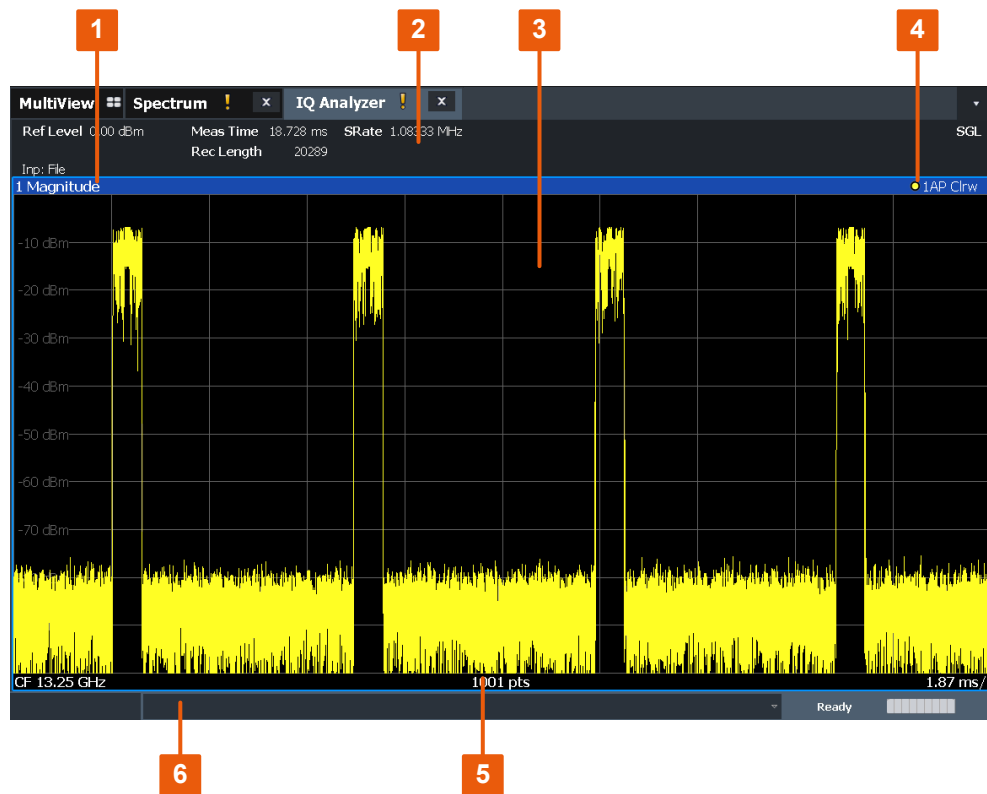
Figure 2-1: Screen elements in the I/Q Analyzer application
