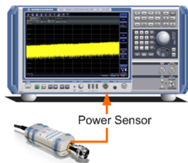
Figure 6-2: Connecting a power sensor using the POWER SENSOR interface
