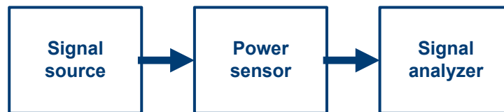
Figure 6-2: Power sensor support – standard test setup
