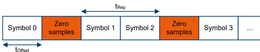
[Figure 2-10: OFDM symbol sequence with zero padding samples](#)
