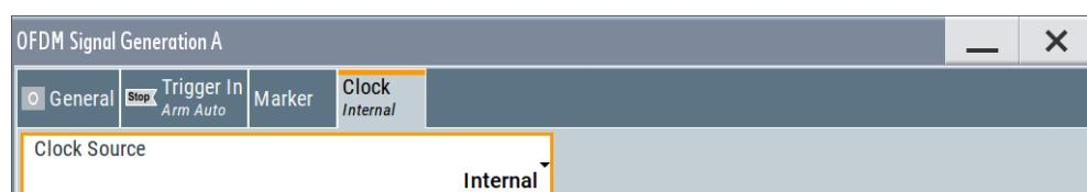
This tab provides settings to select and configure the clock signal, like the clock source and clock mode.
