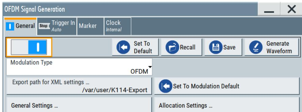
This dialog provides the standard general settings, to the default and the "Save"/"Recall" settings, as well as selecting the modulation type and access to dialogs with further settings.
