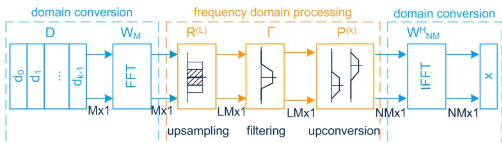
**Figure 2-1: Optimized GFDM transmitter model (from [1])**
