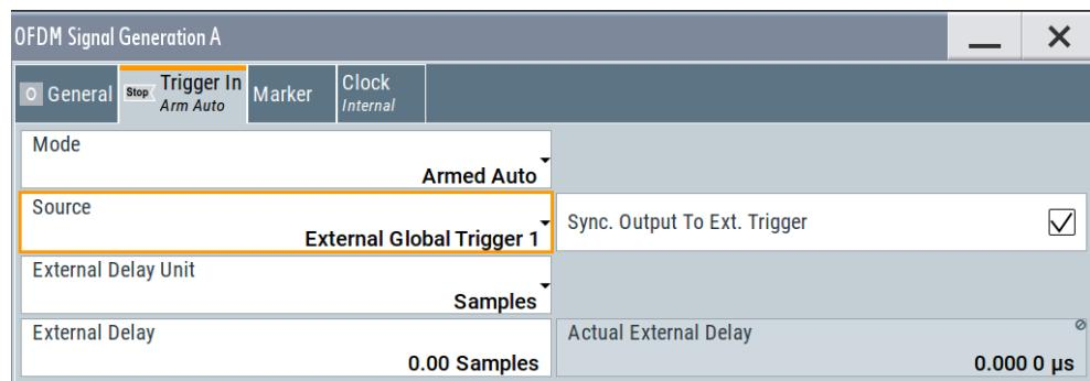
This tab provides settings to select and configure the trigger, like trigger source, trigger mode and trigger delays, and to arm or trigger an internal trigger manually. The header of the tab displays the status of the trigger signal and trigger mode. As in the tabs "Marker" and "Clock", this tab also provides access to the settings of the related connectors.
