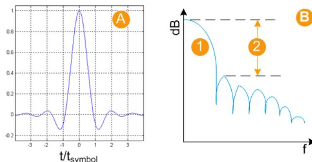
**Figure 2-4: Example of filer characteristics: Root cosine filter with Roll Off Factor = 0.5**
