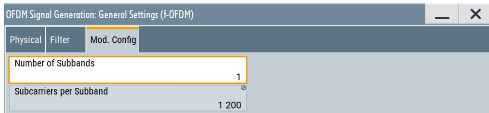
This tab provides settings to configure the modulation for modulation types "f-OFDM", "UFMC", "FBMC" and "GFDM". The provided settings depend on the selected modulation type.
