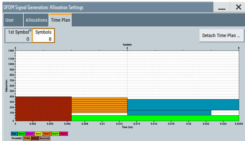
The tab provides a time-frequency resource grid representation of configured allocations. The x-axis shows the time domain in milliseconds (lower axis) or in number of symbols (upper axis part). The y-axis shows the frequency domain with the number of occupied subcarriers as the smallest frequency granularity.
