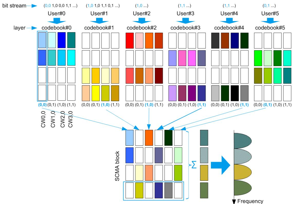
**Figure 2-9: SCMA encoding example ( $K = 4, N = 2, J = 6$ )**
