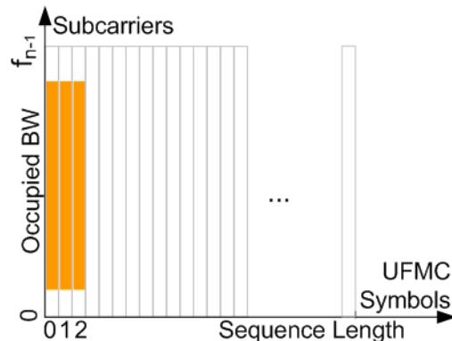
The remaining symbols are filled with the data source and modulated as selected with the parameters [Data Source](#) and [Constellation](#). To set the preamble length, use the parameter [No. Sym..](#)
