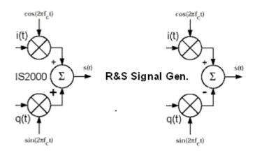
Figure 2-7: Definition of I/Q modulator in IS2000 and the R&S SMBV100B
