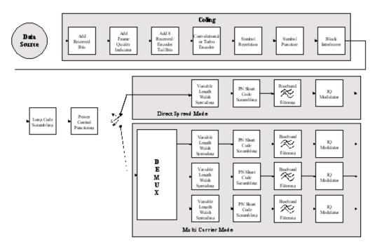
Figure 2-2: Components of the CDMA2000 transmission system in the uplink (reverse)
