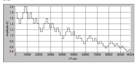
Figure 3-3: Dynamic change of channel power (continuous)
