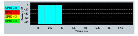
The X axis is the length of the set packet interval in ms, i.e. the duration of the transmission of an encoder packet.
