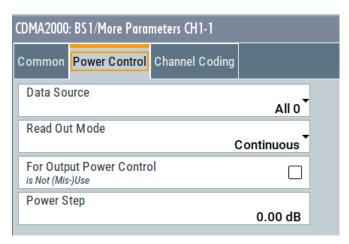
This section contains the parameters required for configuring the power control for the channel types F-FCH and F-DCCH.
