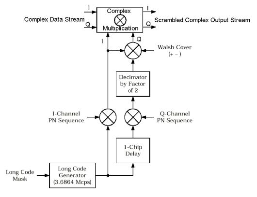
Figure 2-6: Scrambling in the uplink RC3, RC4 and RC5
