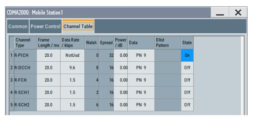
This table contains the channel table for configuring the channel parameters individually.
