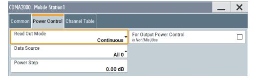
This dialog contains the parameters for configuring the power control bits for mobile stations.
