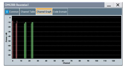
This tab graphically shows the active code channels. The channel number is plotted on the X axis. The red bars represent the special channels, the green bars the traffic channels. The channel index is plotted on the X-axes. The height of the bars shows the relative power of the channel.
