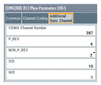
This section contains the additional parameters for the channel type F-SYNC.
