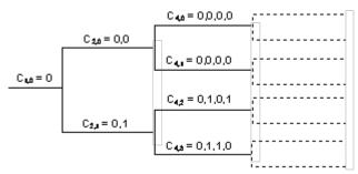
To find a 3GPP code that corresponds to a CDMA2000 code, the bit-inverted line (line index) has to be selected in the 3GPP matrix of identical spreading factor.
