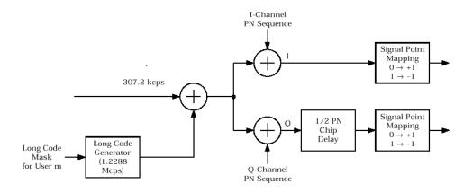
Figure 2-4: Scrambling in the uplink RC 1 and RC2
