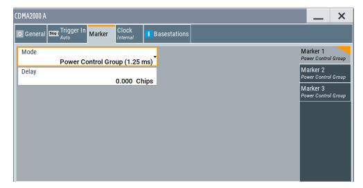
This tab provides settings to select and configure the marker output signal including marker mode and marker delay.
