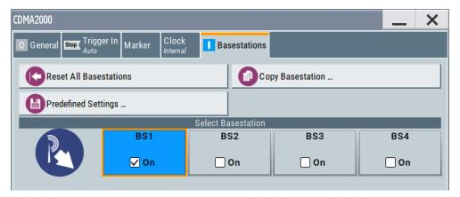
This dialog provides access to the appropriate settings dialogs for configuring the base stations.
