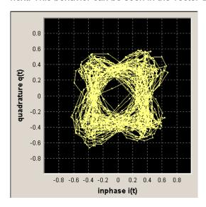
Figure 2-5: Scrambling in the uplink RC 1 and RC2
