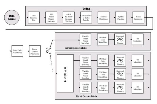
Figure 2-1: Components of the CDMA2000 transmission system in the downlink (forward)
